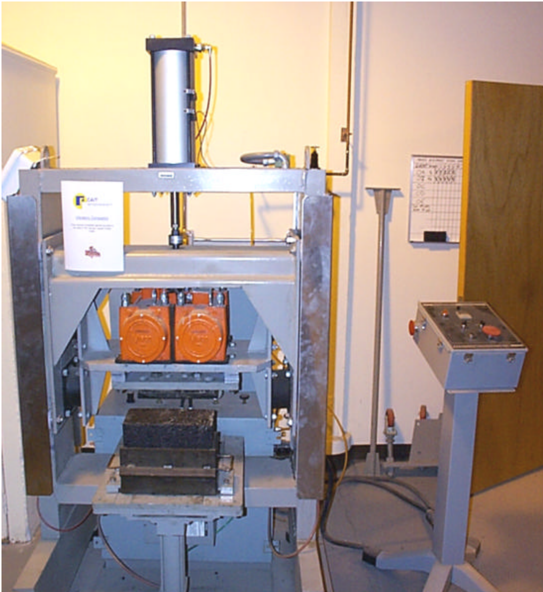
Figure 4 – Vibratory Compactor at RAPL
