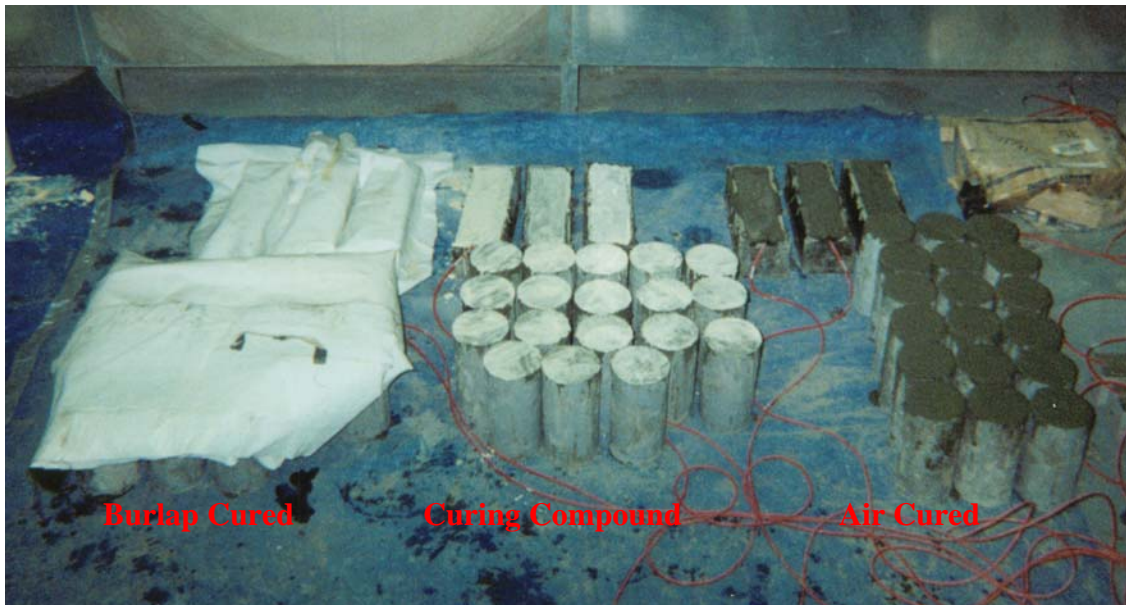
Figure 2. Concrete cured using different curing methods
