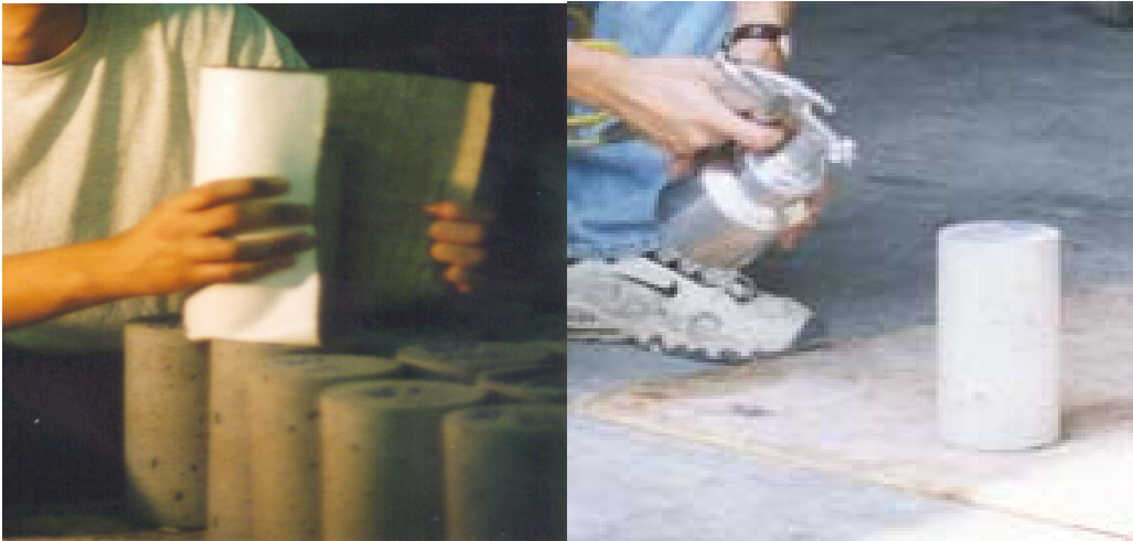
Figure 16. Method of applying burlap and curing compound on to specimens
