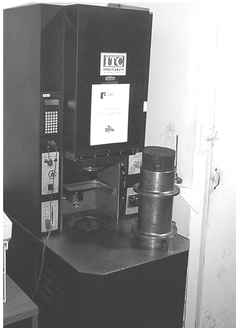
Figure 17 – Superpave Gyratory Compactor at RAPL (Manufactured by Interlaken Technologies)
