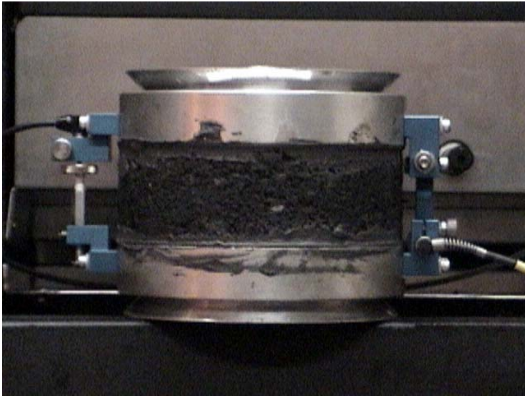
Figure 8 – SST Specimen Glued to Caps with LVDT's Attached
