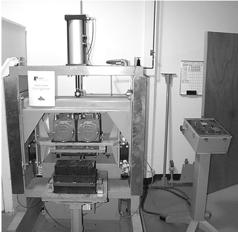
Figure 18 – Vibratory Compactor at RAPL (Manufactured by Pavement Technologies Inc.)
