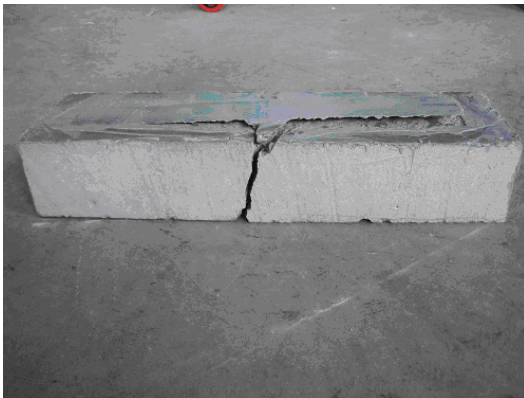
(a) & (b) Debonding of CFRP without wrap (beam7).
