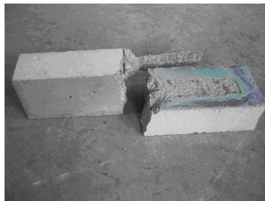
(a) & (b) Debonding of CFRP without wrap (beam7).
