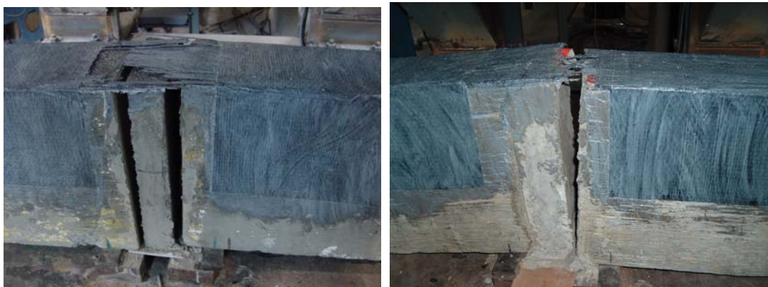
Figure 89. CFRP rupture of beams 17 (left) and 18 (right).
