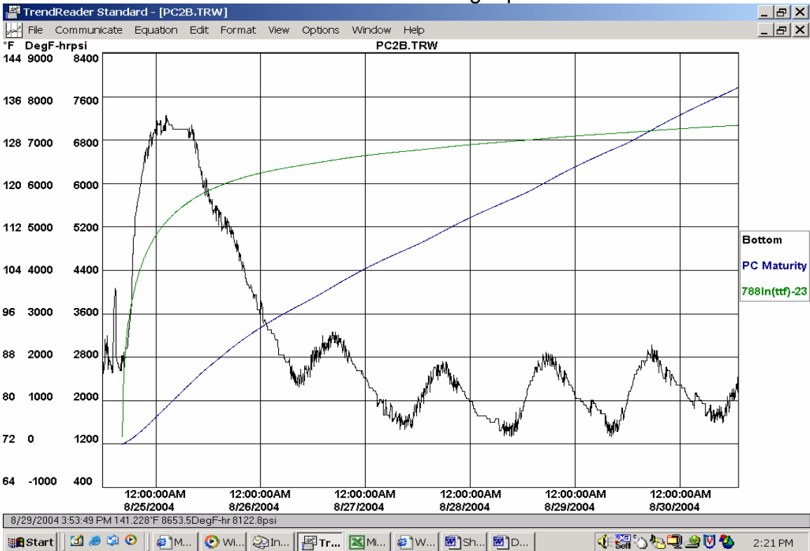
Beam 2 south critical strength prediction
