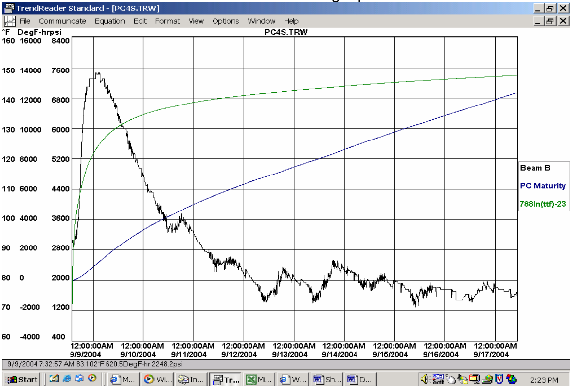
Beam 4 south critical strength prediction
