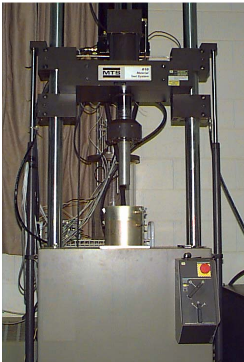
Figure 15 – Testing Set-up Used for the CBR Testing
