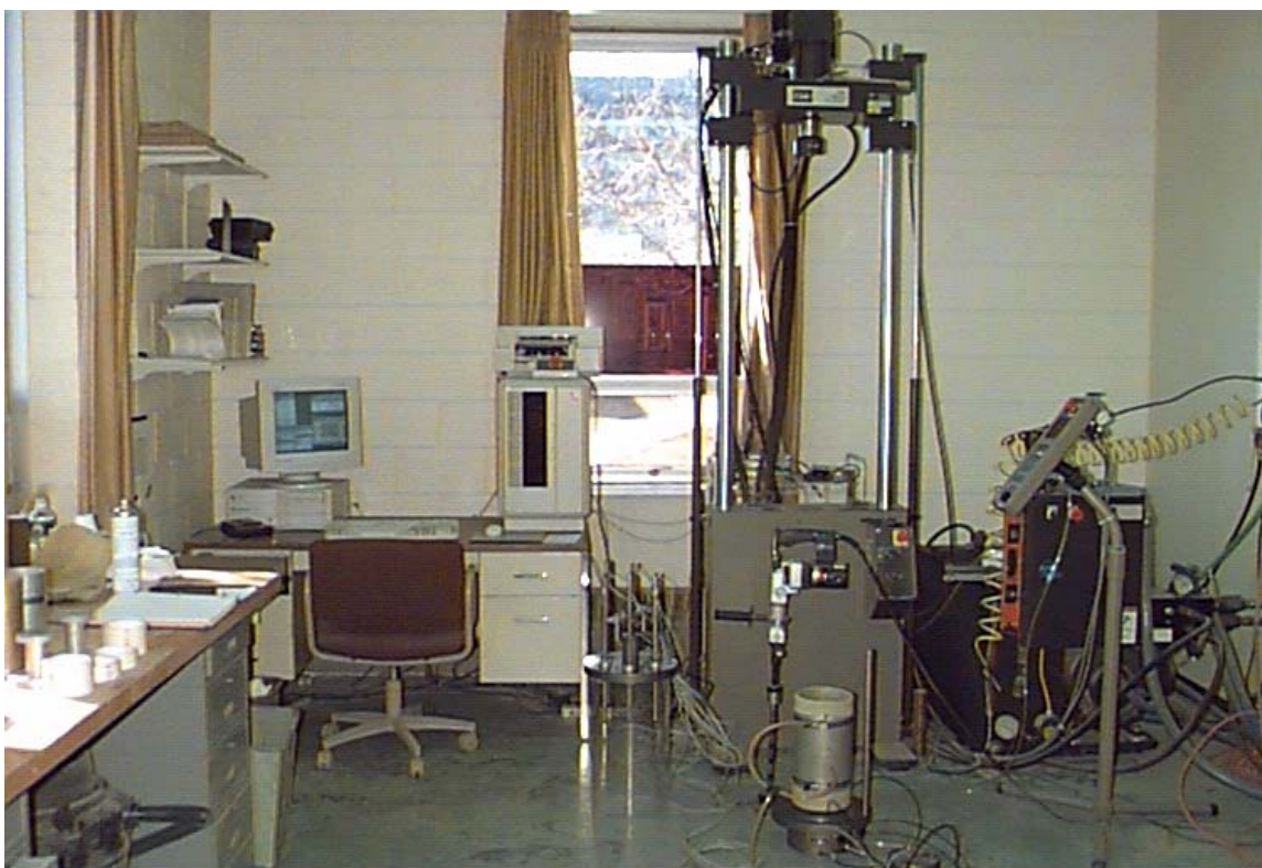
Figure 25 – Test Set-up Used to Conduct Resilient Modulus Testing
