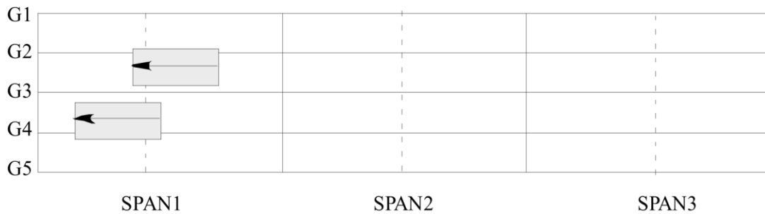
Figure 30. GDF obtained at a distance of 64 ft from abutment of Stage I construction when Trucks A1-1 and A1-2 are following or staggered
