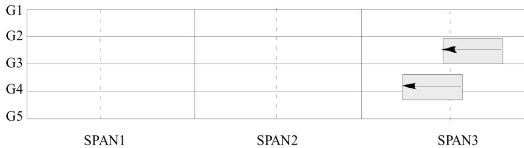
Figure 32. GDF obtained at a distance of 378 ft 11 in. from abutment of Stage I construction when Trucks A1-1 and A1-2 are following or staggered
