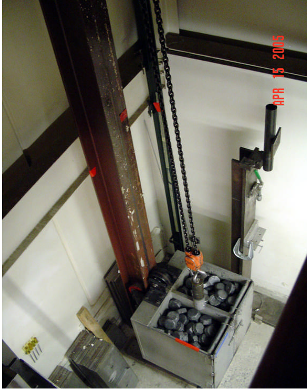
Figure 12 a&b. Drop test apparatus without a test unit, and with TMA installed. (Enidine)
