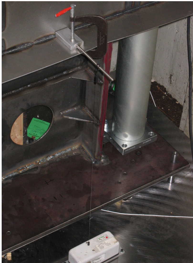
Figure 14. String pot set up to measure displacement and velocity. (Enidine Inc.)
