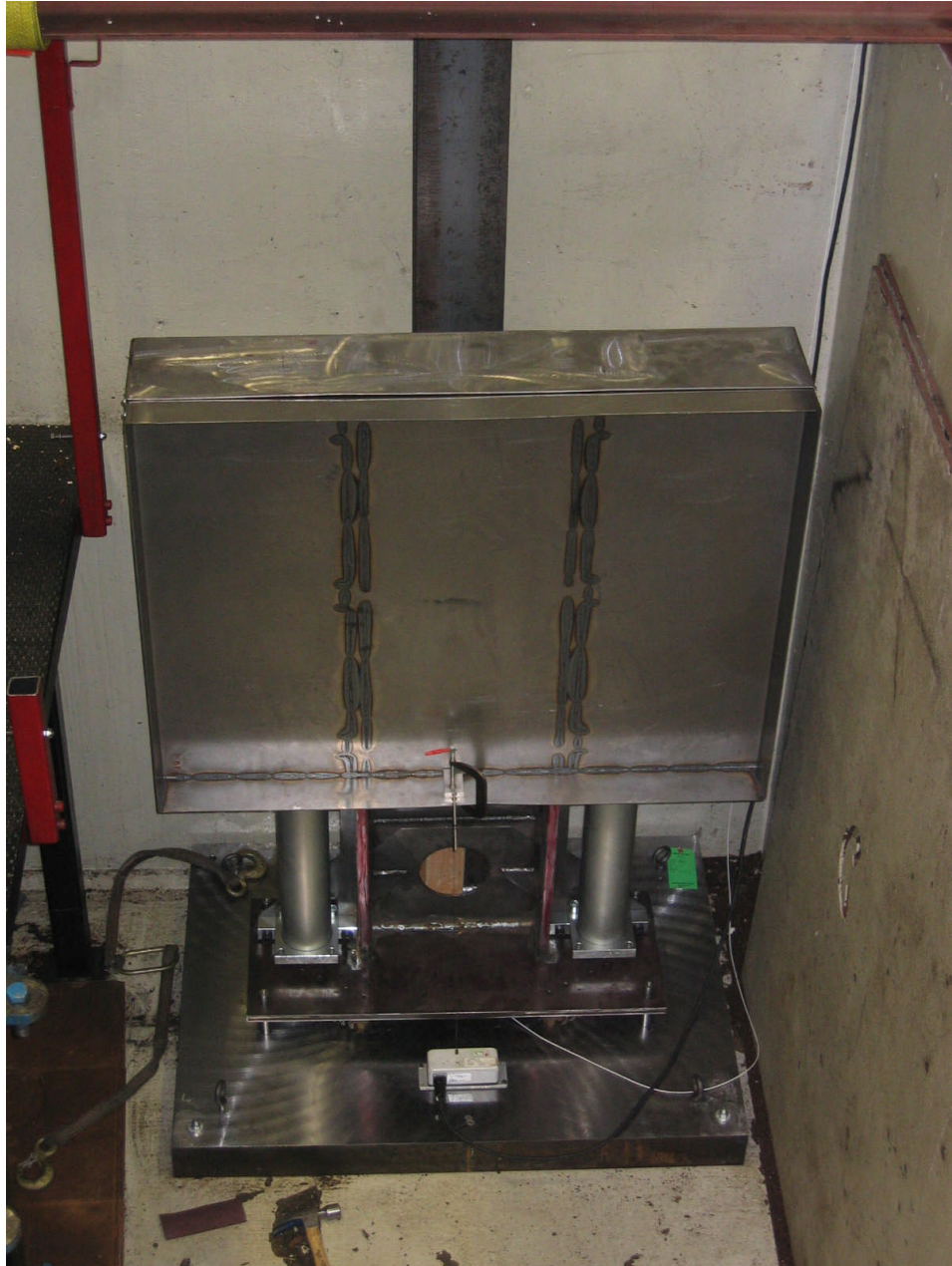
Figure 11. Fabricated TMA quarter-scale test unit, installed in drop test apparatus.
