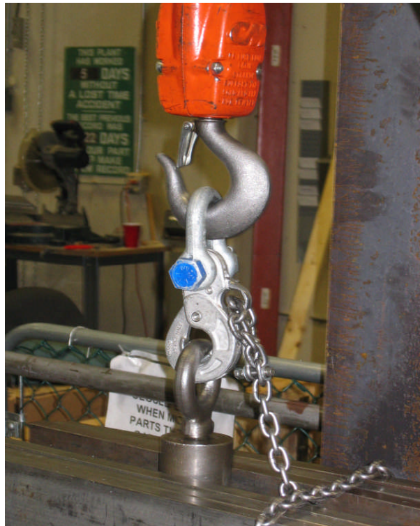
Figure 13 a&b. 4,000 lb drop weight and quick release hook (Enidine Inc.)
