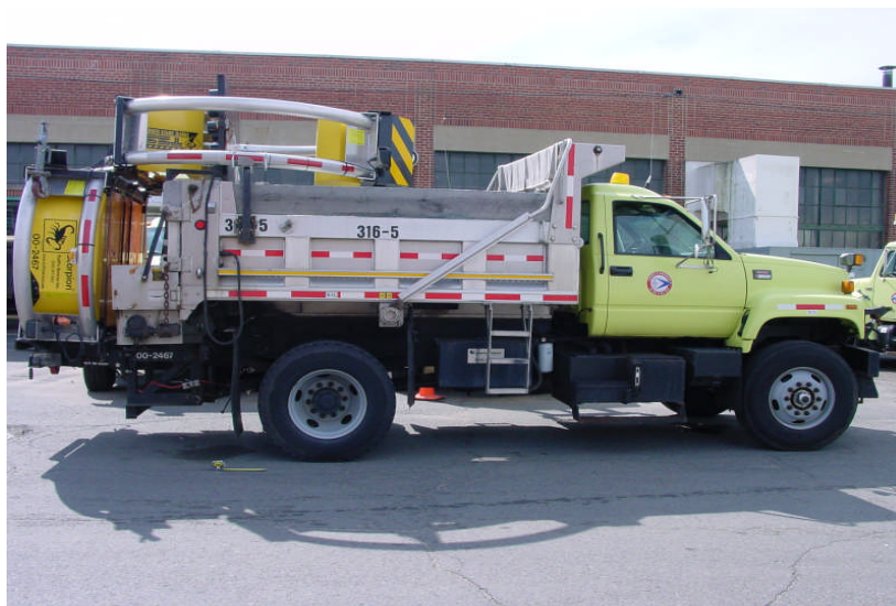
Figure 1. Standard dump truck used for TMA support.
