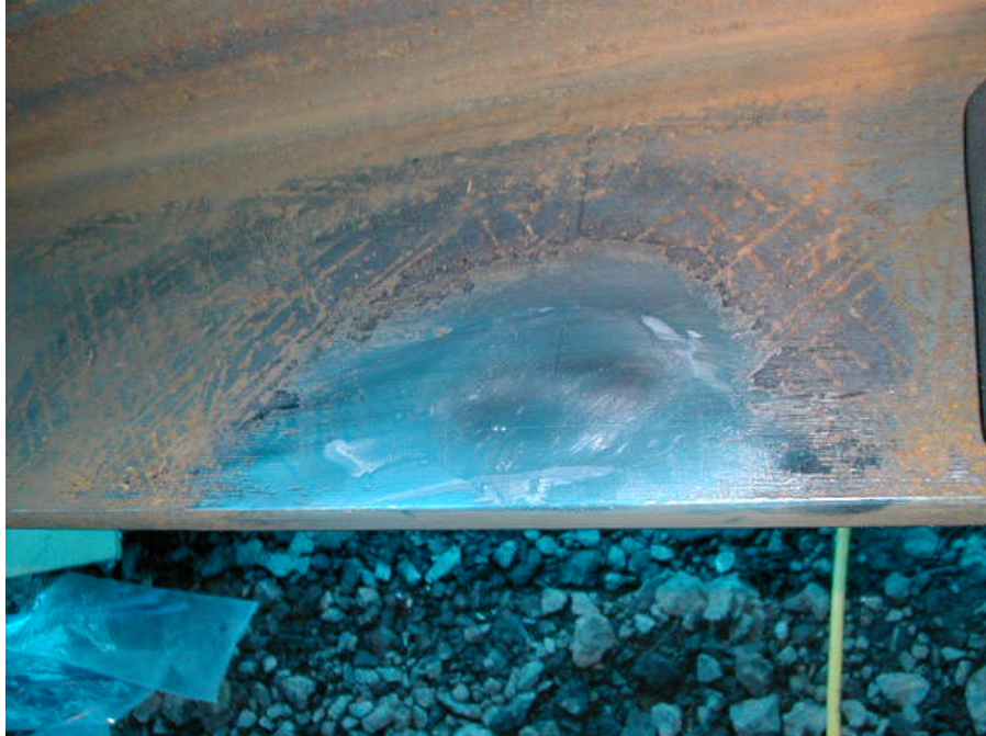
Figure 21. Burnishing the surface using a pencil, at the location of gage installation.
