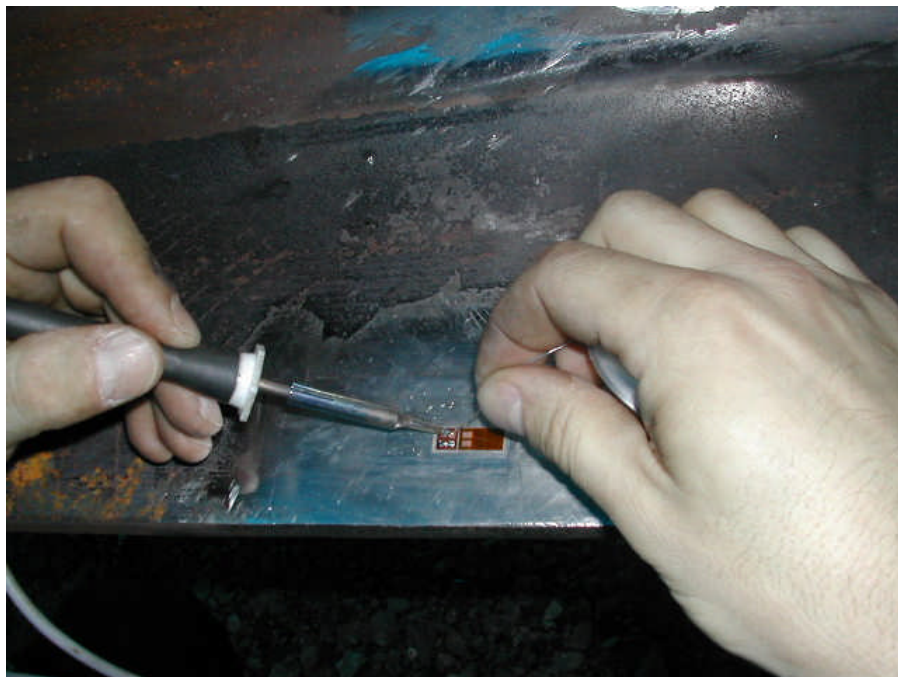
Figure 34. Sauter magnet wires on the strain gage
