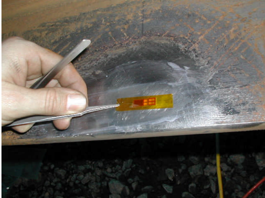
Figure 23. Installing the strain gage
