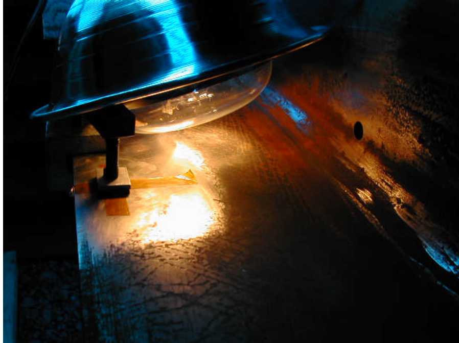
Figure 29. Curing the strain gage under heating lamps.
