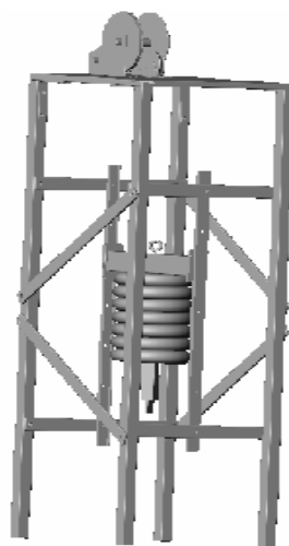
Figure 8-4. Impact Penetration Test Apparatus
