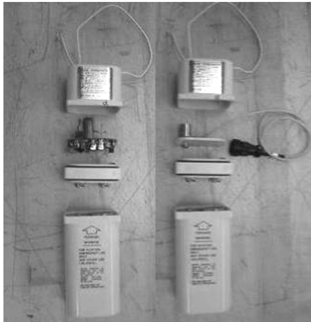
Figure 9-11. ELT retrofitted with a Laboratory Grade Accelerometer
