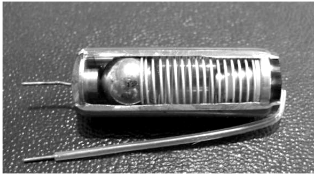
Figure A-9. Cut-away of E-01 G-switch
