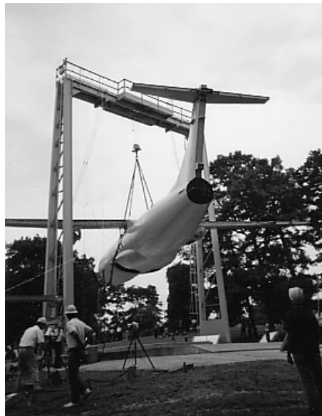
Figure 8-12. ATR42-300 Elevated for Drop Test
