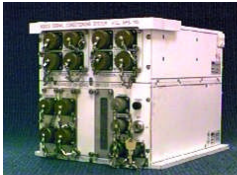
Figure 49: A D v a n c e d O n b o a r d C o m p u t e r S y s t e m (ADOCS)
