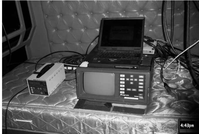
Figure 3: ROVER system used for measuring and recording emissions during HDDV idling conditions.
