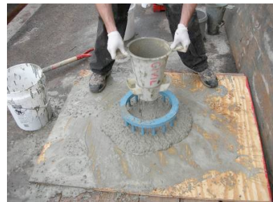
Figure 2. J-Ring Flow Test
