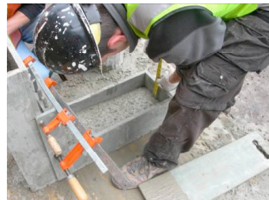
Figure 4. L-Box Test Measurement h2
