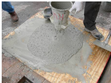
Figure 1. Slump Flow Test
