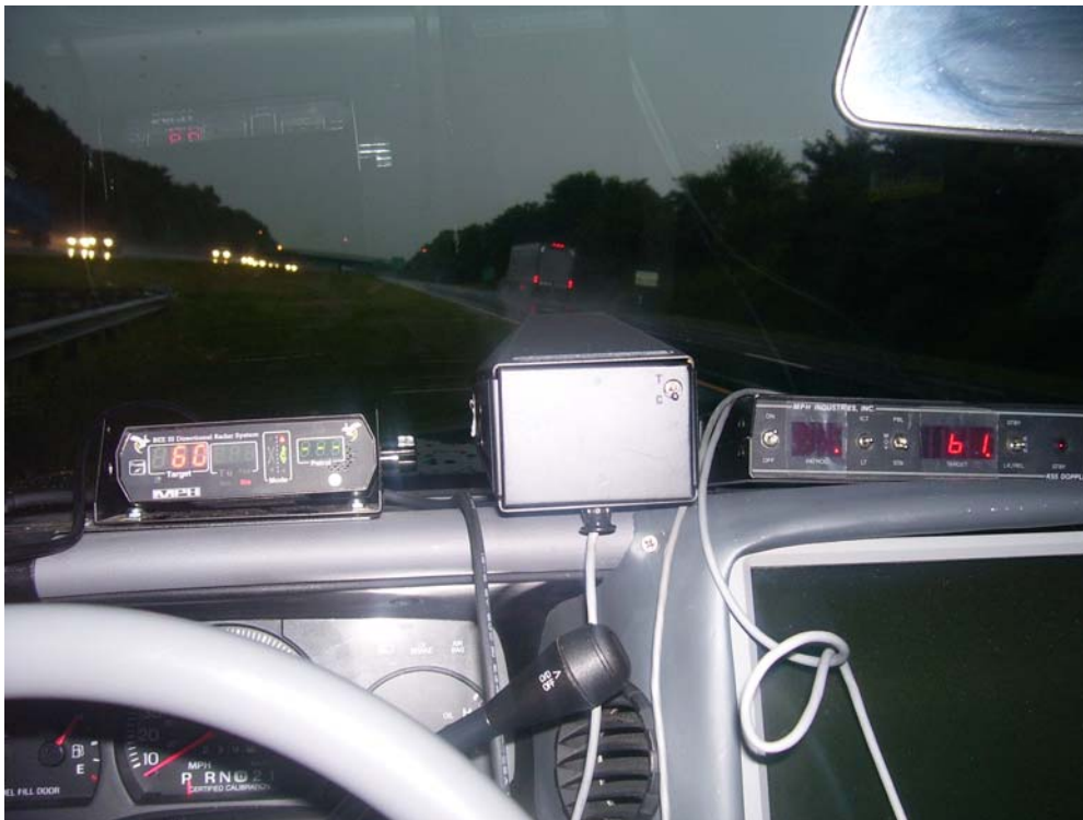
Figure A.2 Test radar units mounted on dashboard
