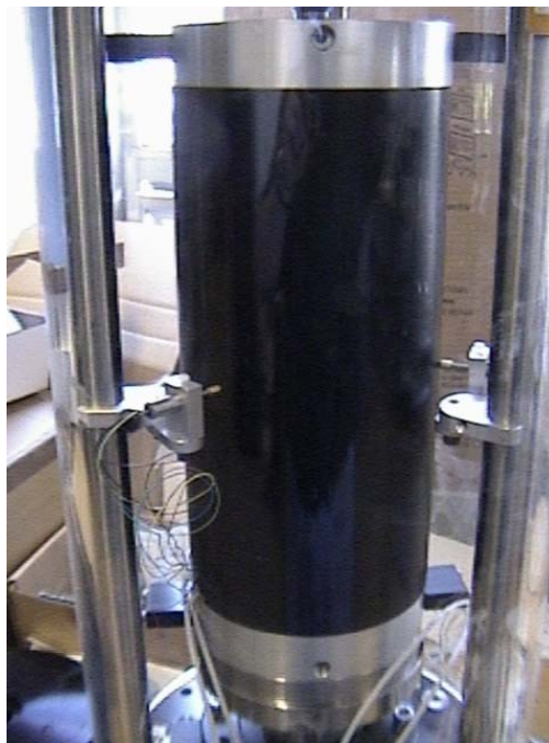
Figure 2 – Resilient Modulus with Radial LVDT Test Set-up
