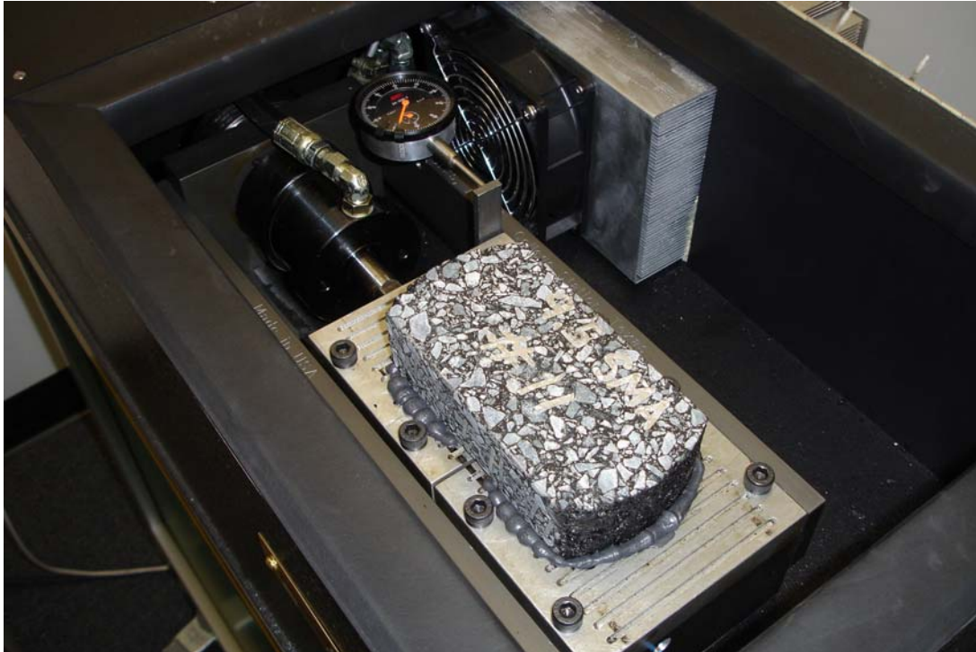
Figure 22 – Picture of the Overlay Tester (Chamber Door Open)
