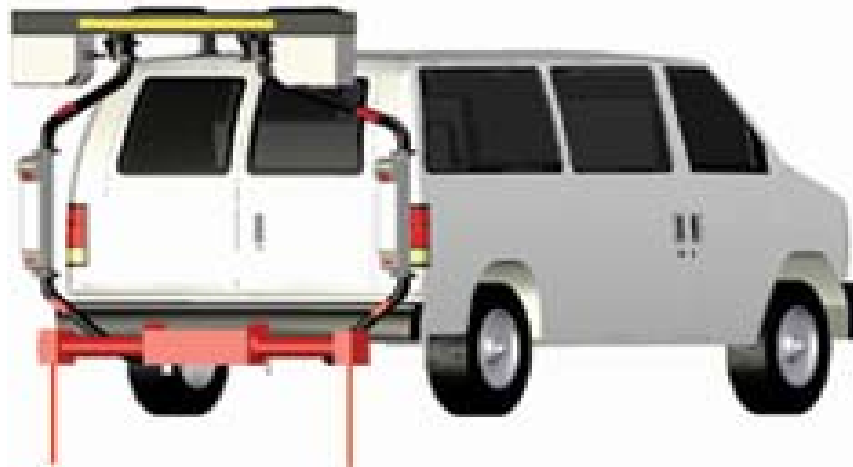
Figure 10: Mandli Road Surface Profile (RSP)
