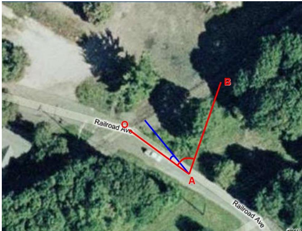
Figure 42. Computed deflection angle based on safe distances standards (red) vs. actual visibility deflection angle (blue)
