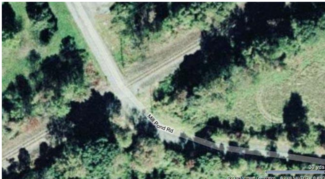
Figure 41. Railroad crossing with obstructed field of view in Washington Twp., NJ
