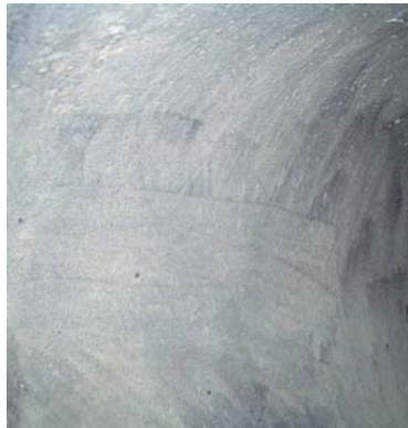
Figure 5. Clay surface coated with inorganic polymer composite
