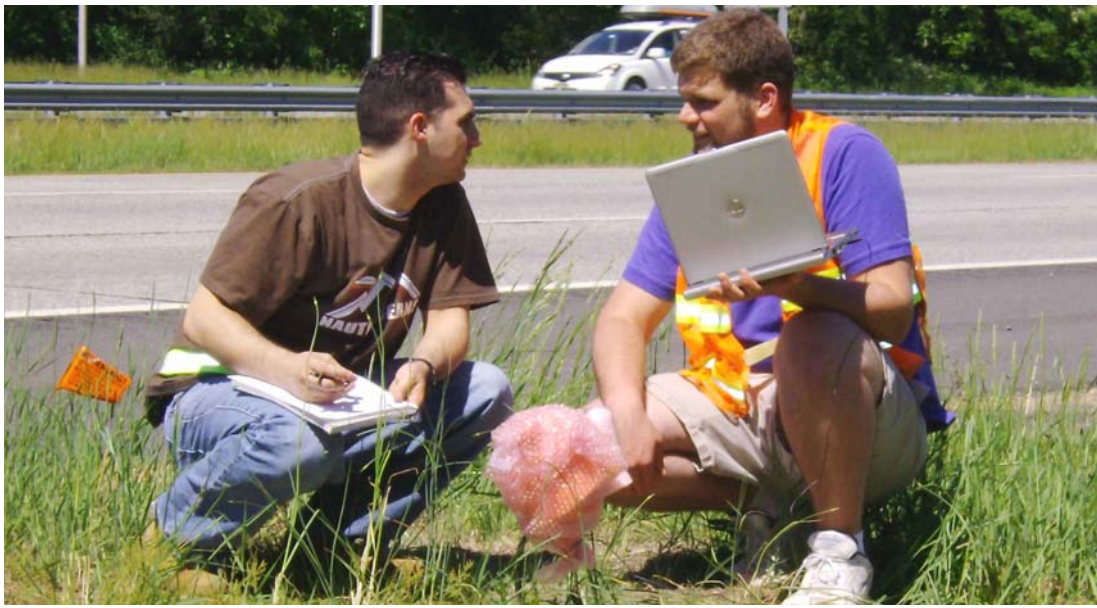
Figure 3: Laptop computer and microphone (center) used to detect acoustic signals
