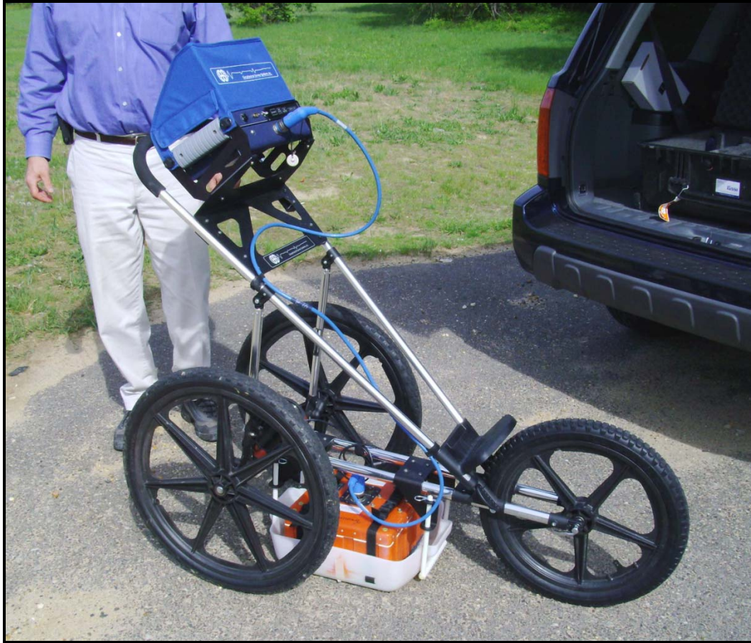
Figure 25 – A typical GPR looks and is pushed similar to a lawnmower.
