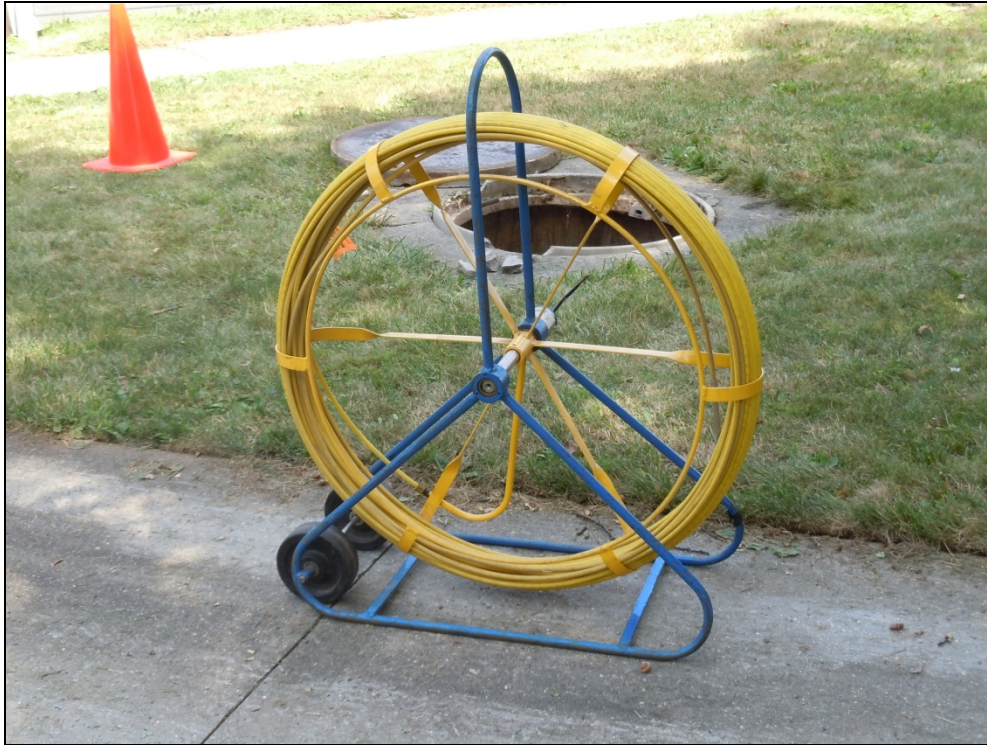
Figure 3 – Snake like device that can functions as a TW in conduit that has none.
