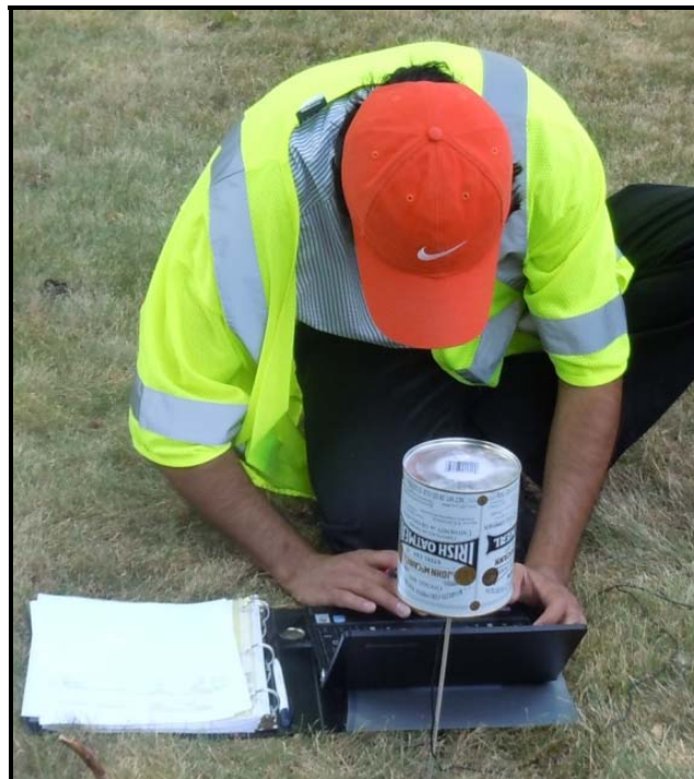
Figure 16 - Microphone and receiver (laptop/sound card with spectrum analyzer software)
