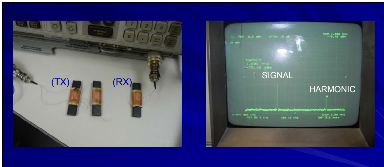
Figure 13 – Test of diode based RFID system for improved TW.
