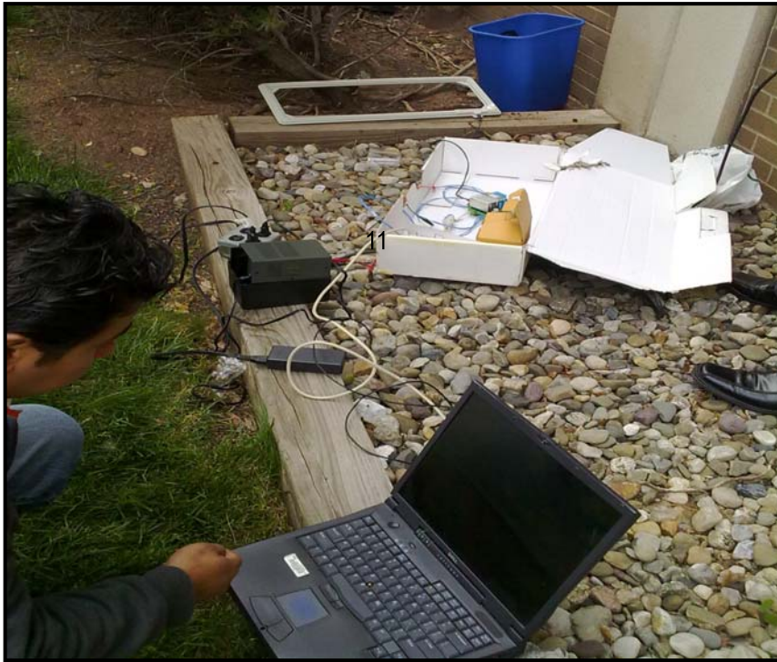
Figure 11 – Test of RFID TAG system (134.2 kHz) when buried in the ground
