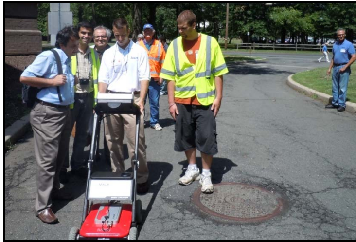
Figure 1 – Mala GPR test over asphalt at DOT headquarters.
