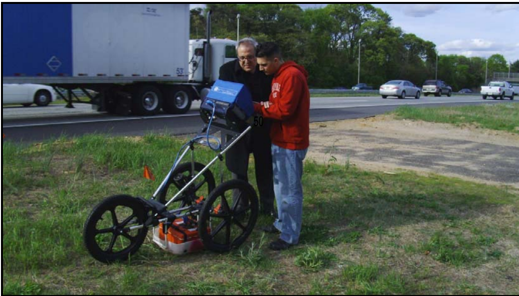
Figure 3: GPR in test operation.
