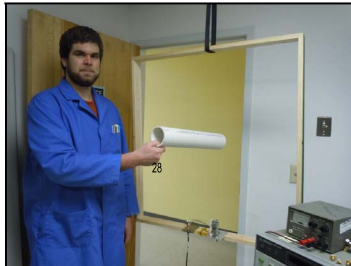
Figure 30 – Electro-magnetic impedance measurement techniques were found ineffective with fiber conduit.
