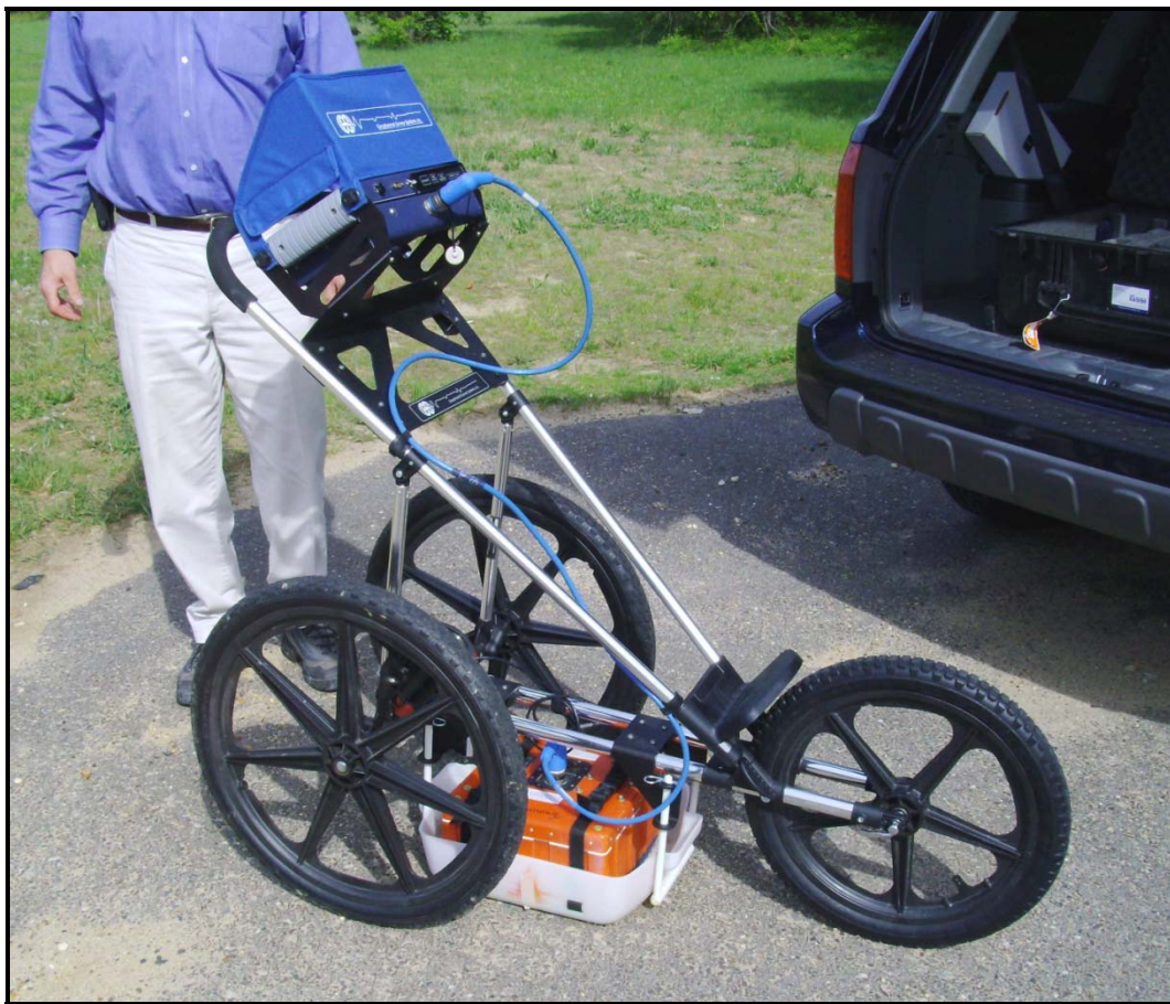
Figure 1: The GSSI GPR is pushed similar to a lawnmowers
