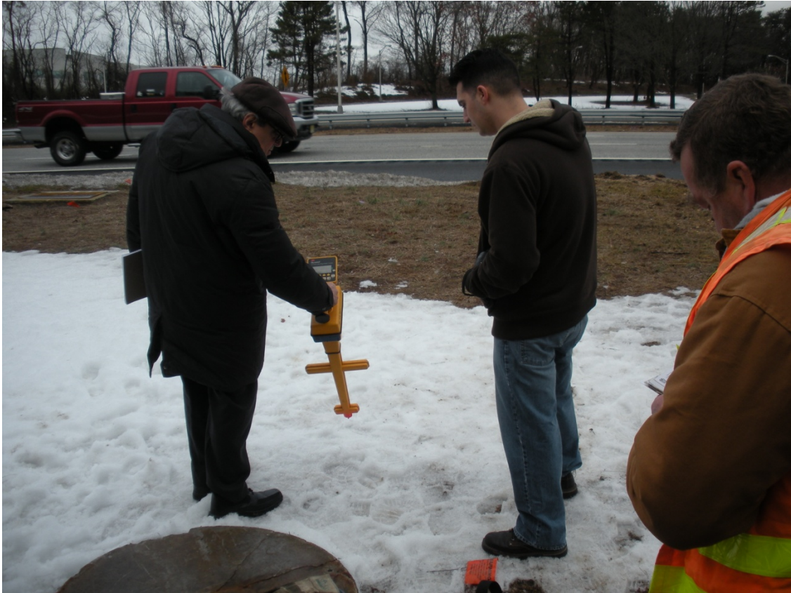
Figure 5: Trace wire receiver being used to detect conduit. The trace wire's signal could be clearly detected.
