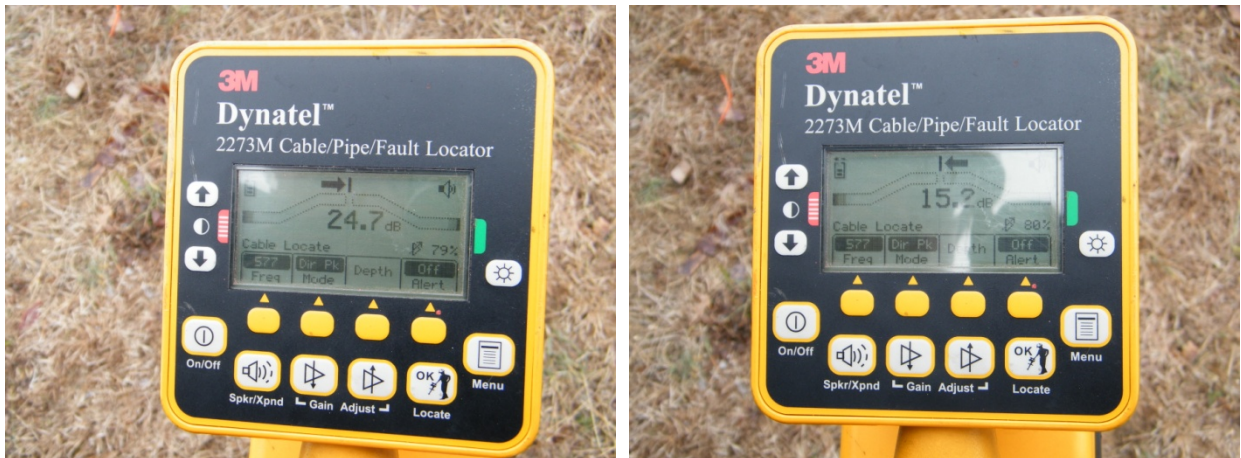
Figure 6: Trace wire receiver display shows an indication of signal level and wire location.
