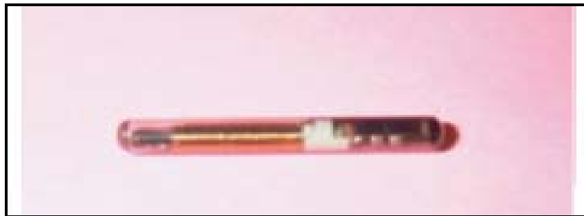
Figure 9 - Typical RFID tag based on near field coupling at 128 kHz, 1 cm in length. [Trovan RFID, "Method and apparatus for modulating and detecting a sub-carrier signal for an inductively coupled transponder," www.trovan.com , US patent # 5,095,309].
