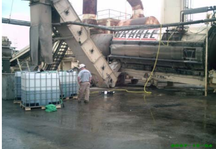
Figure 2. Evotherm Added to Drum (85% Water; 15% “Chemical Package”)
