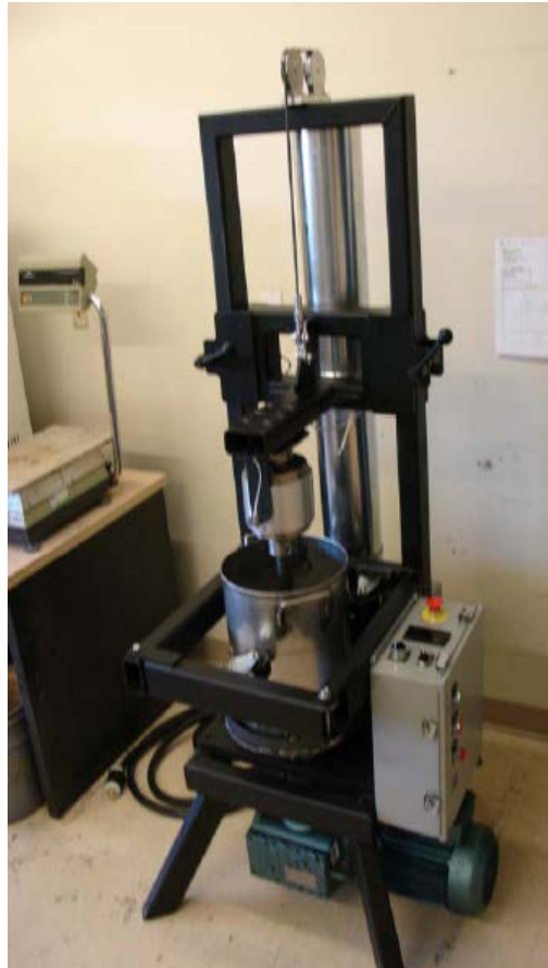
Figure 21. Asphalt Workability Device Developed by the University of Massachusetts, Dartmouth
