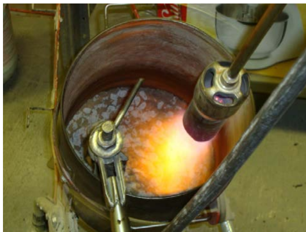
Figure 15. Heating and Mixing Aggregate Blend
