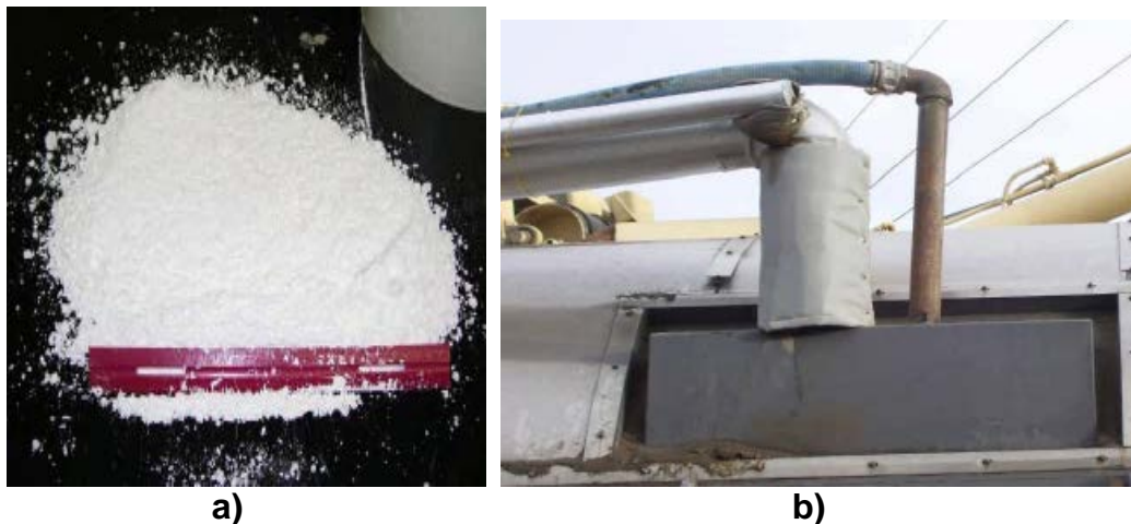
Figure 6. a) Advera type of Synthetic Zeolite and b) Feeding Port for Zeolite Into Drum Plant
