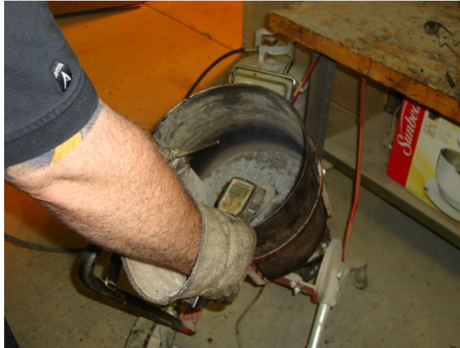
Figure 16. Monitoring Temperature of Aggregate Blend with Infrared Temperature Probe
