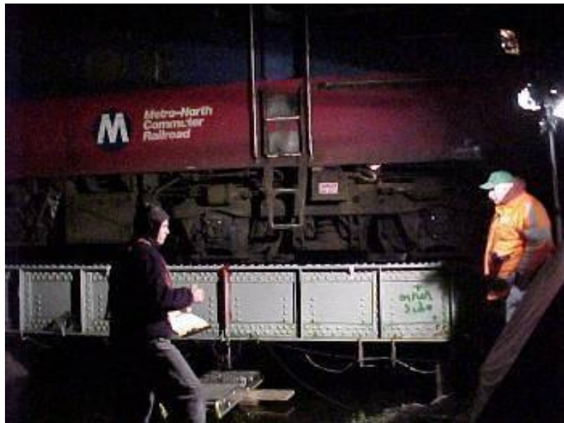
Figure 9. Train positioned for static test (11)
