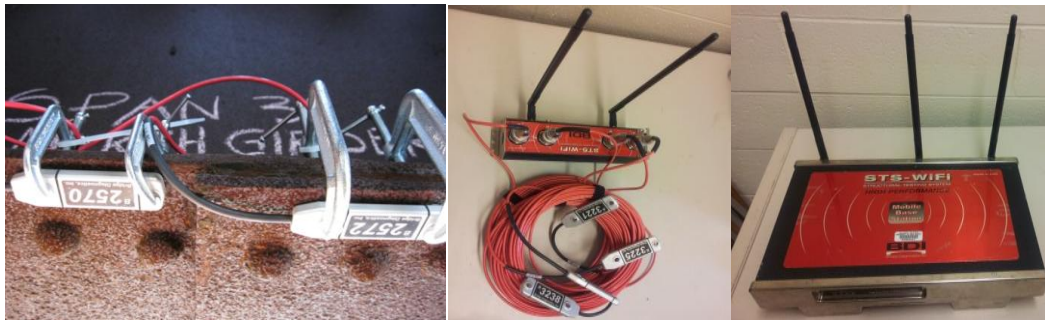
(a) (b) (c) Figure 25. (a) STS strain transducer; (b) junction node, and (c) main unit
