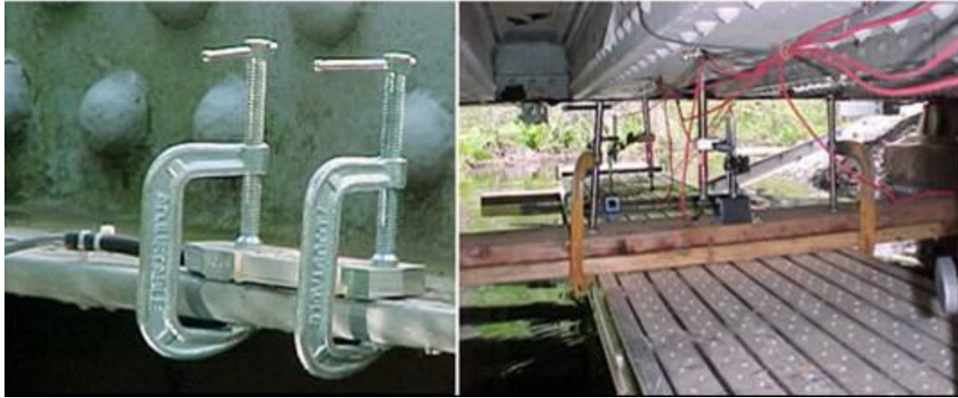
Figure 8. Sensors used to measure strains and deflection (11)
