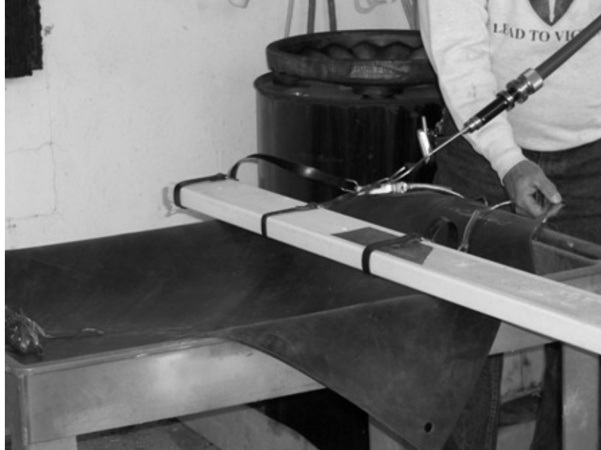
Figure 45. Doble testing of gate arm
