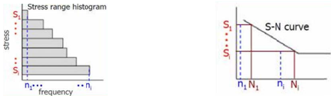
Figure 49. stress range spectrum and S-N curve to find out the cumulative damage due to each stress range.
