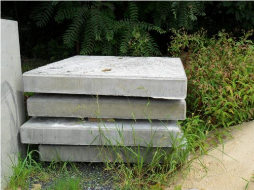
Figure 12. Items precast using recycled concrete aggregates
