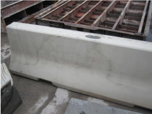
Figure 12. Items precast using recycled concrete aggregates
