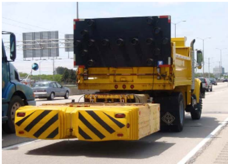
Figure 2. A typical truck-mounted attenuator and arrow board used for moving lane closures (9)
