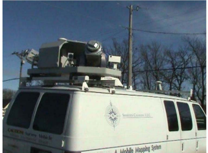
Figure 25. Mobile LiDAR Scanner for surveying (49,50)
