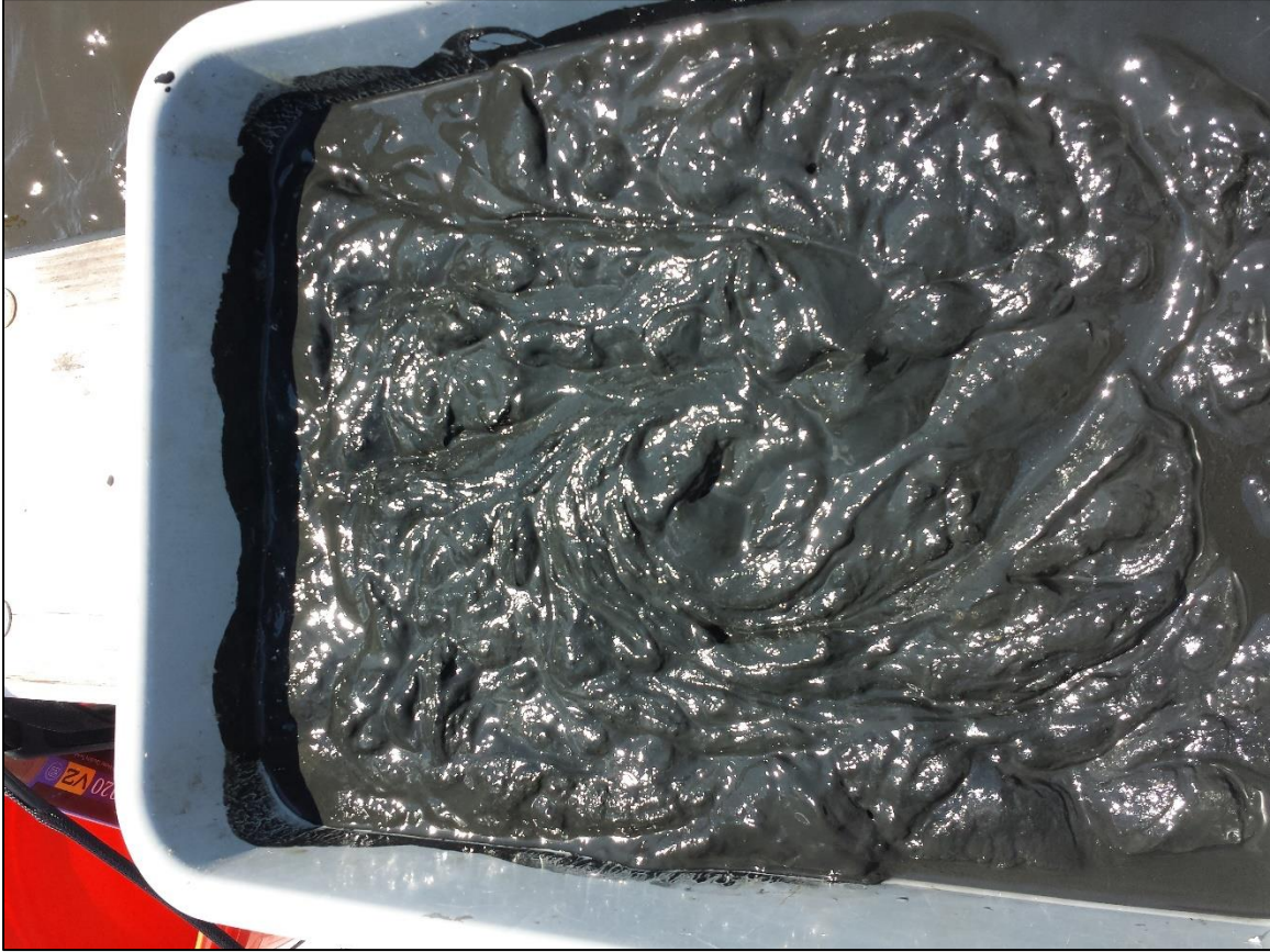
Figure 30, The grab sample from the center of Dredged Hole 93 consisted of dark grey silt with some detritus, and black or dark grey silt.
