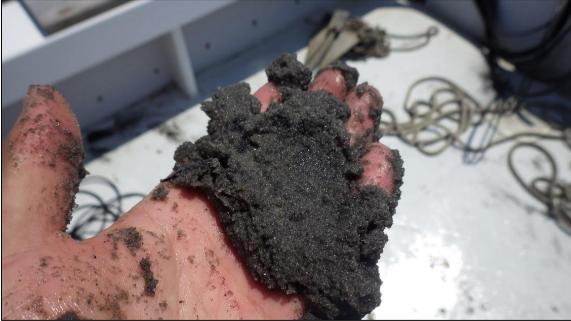
Figure 7, The shallow control sample (depth of 1m) for Dredged Hole 18 contained grey sand with plant debris.
