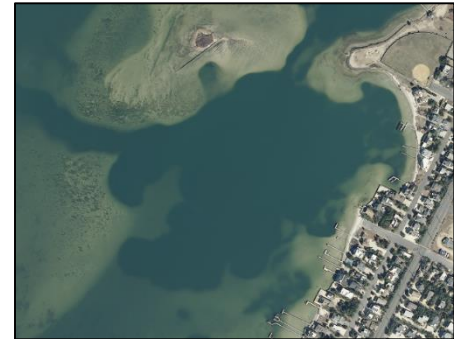
Figure 35, Dredged Hole 54 is clearly depicted in 2012 aerial photography by an irregular delineation with several cusps. A channel connecting the feature to Barnegat Bay is located at the left of the image and a smaller second channel is visible at the top of the image.
