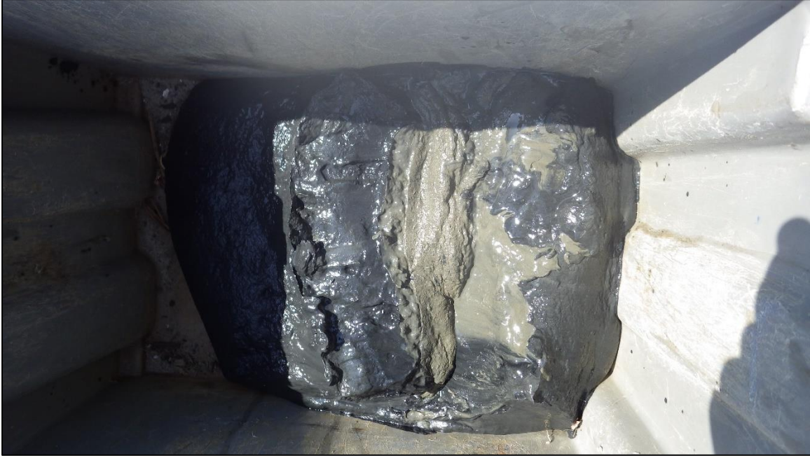
Figure 52, A benthic grab sample from Dredged Hole 85 consisted of black/grey silt with small amounts of sand and no living organisms.
