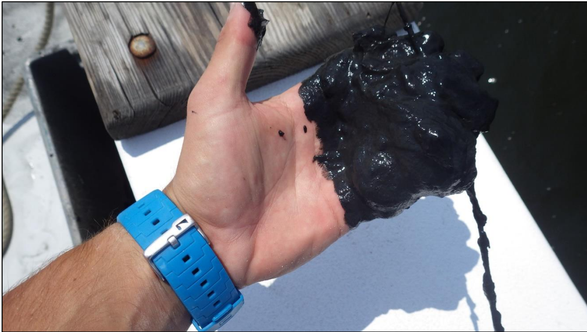
Figure 10, The grab sample from the deepest sampling location in the center of Dredged Hole 25 consisted of black mud and plant debris.
