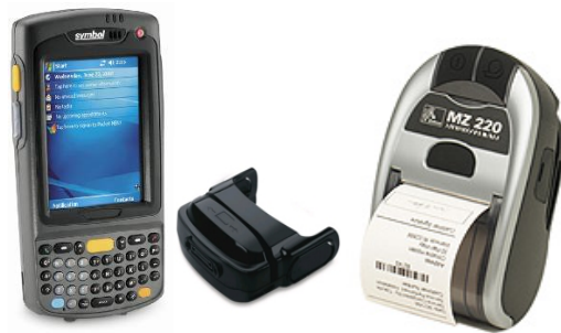
Figure 6. Handheld device components for on-board ticket sale and validation (14)
