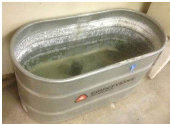
Figure 18 Water Curing Tanks
