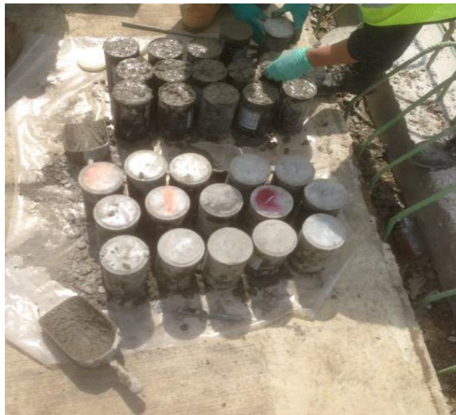
Figure 14. Covering Molds with lids to prevent evaporation
