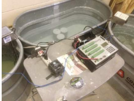
Figure 19 Accelerated (Hot) Lime Bath Curing
