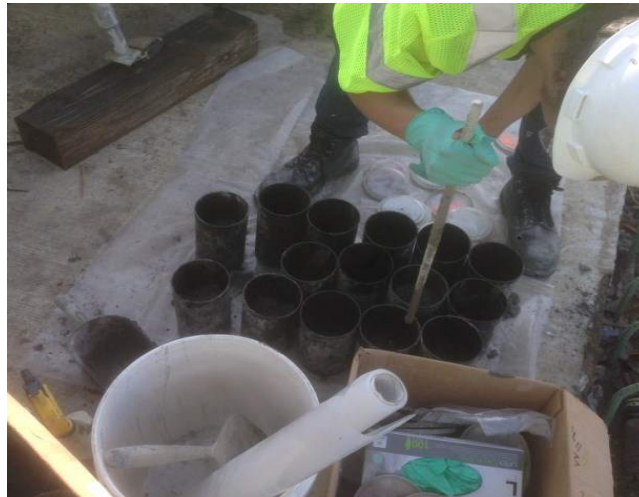
Figure 13. Rodding Fresh Concrete in Molds
