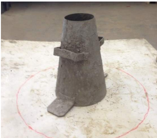
Figure 8. ASTM C134 Slump Test Setup
