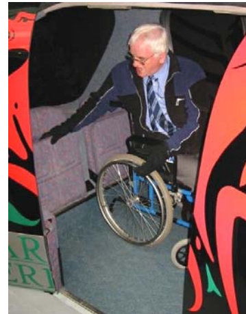
Figure A-14 - ULTra Wheelchair Access Image Courtesy of ATS
