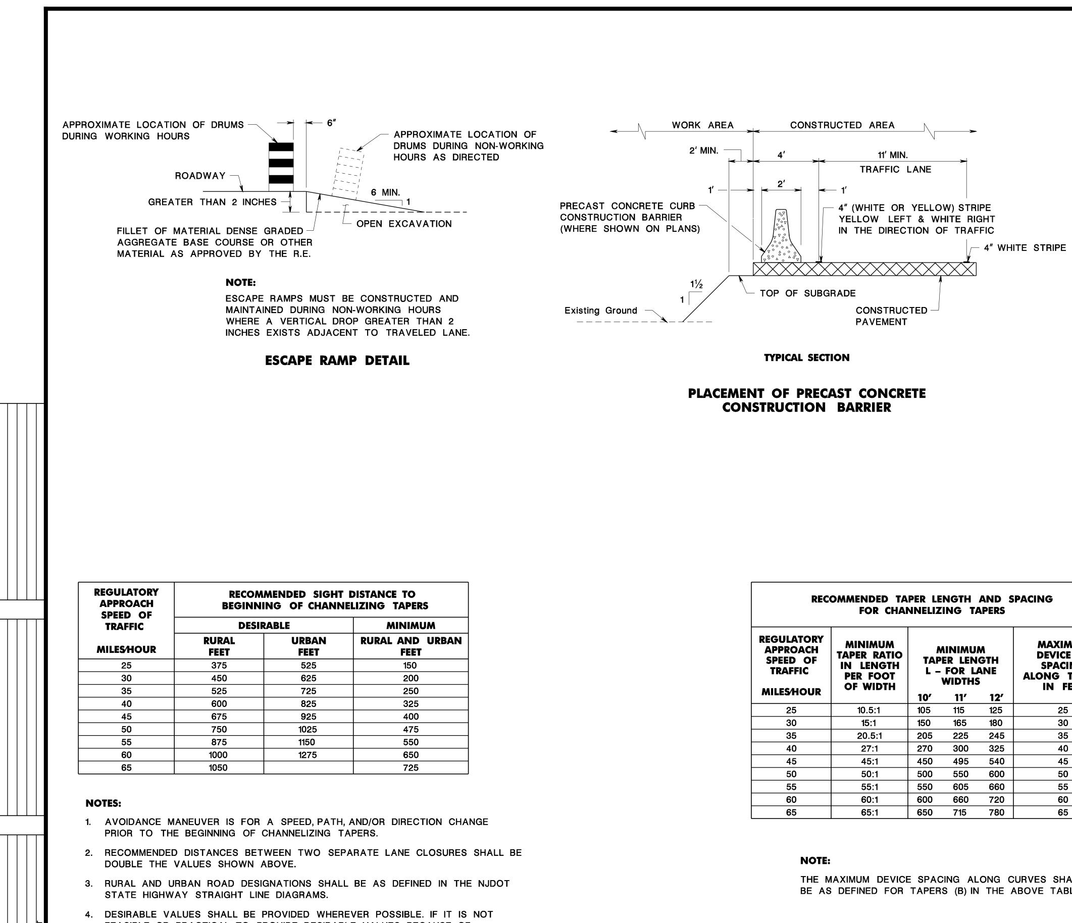
FEASIBLE OR PRACTICAL TO PROVIDE DESIRABLE VALUES BECAUSE OF HORIZONTAL OR VERTICAL CURVATURE OR IF RELOCATION OF THE TAPER IS NOT POSSIBLE, THEN MINIMUM VALUES CAN BE APPLIED. WHEN MINIMUM VALUES ARE USED, SPECIAL ATTENTION SHOULD BE GIVEN TO THE USE OF SUITABLE TRAFFIC CONTROL DEVICES FOR PROVIDING ADVANCED WARNING OF THE CONDITIONS THAT ARE LIKELY TO BE ENCOUNTERED.
