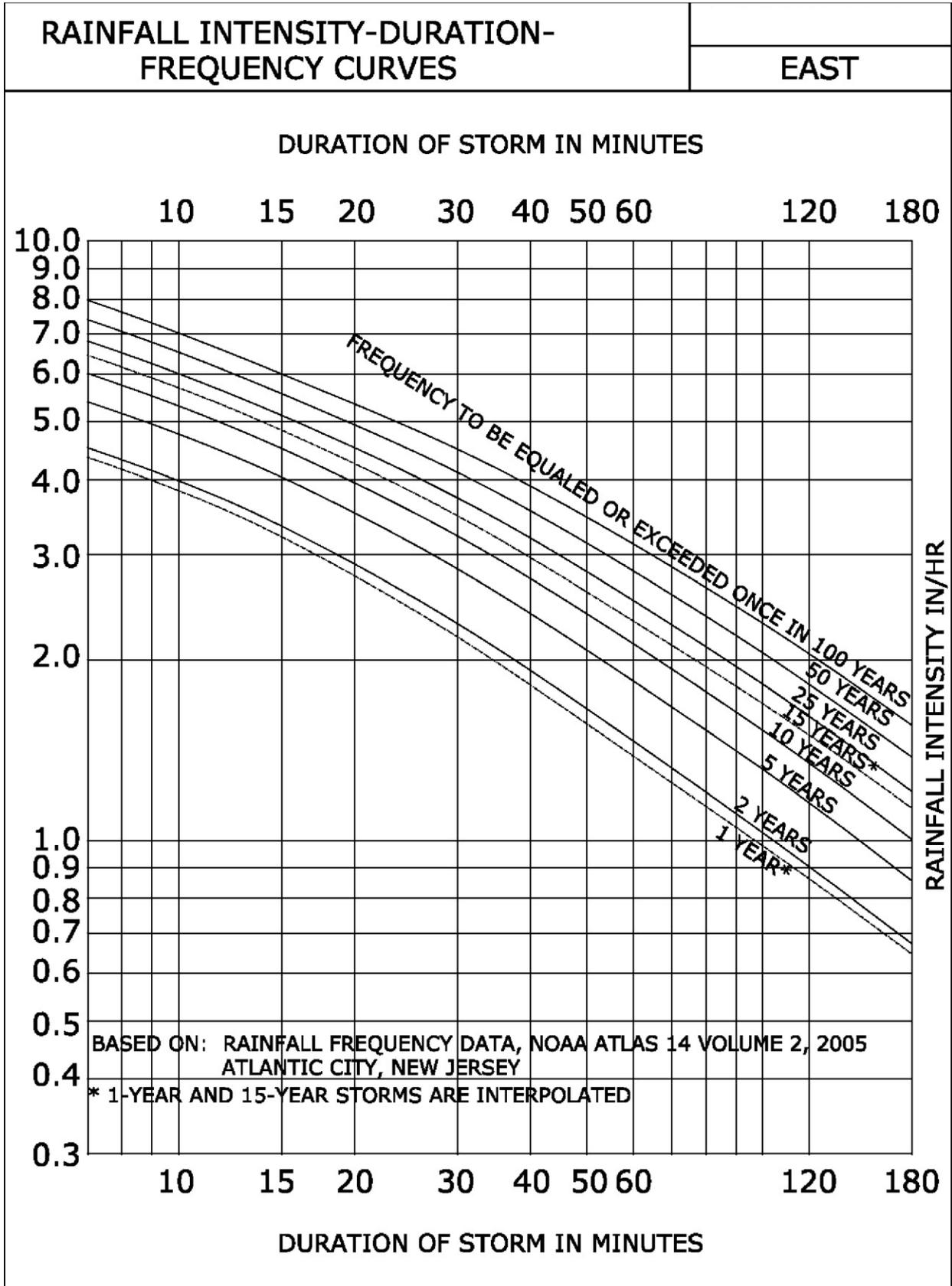
Use of computer program-generated I-D-F curves shall be accepted provided the results match those obtained from Figures 3-2 through 3-4.
