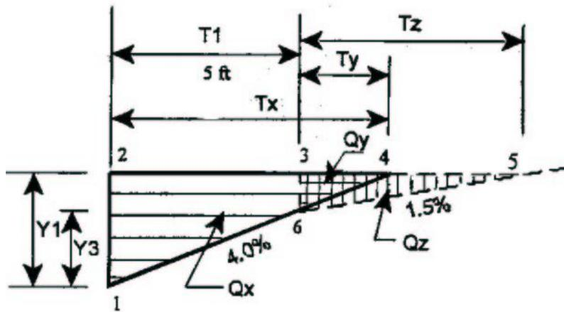
Initially, a depth is assumed ( $y_1$ ).  $Q_x$ ,  $Q_y$  and  $Q_z$  are then calculated using the above equation. The flow contained in the composite section ( $Q_t$ ) is equal to  $Q_x + Q_z - Q_y$ . This process is repeated until  $Q_t = Q$  (actual flow in the gutter).  $T$  (actual spread width) is equal to  $T_x + T_z - T_y$ .
