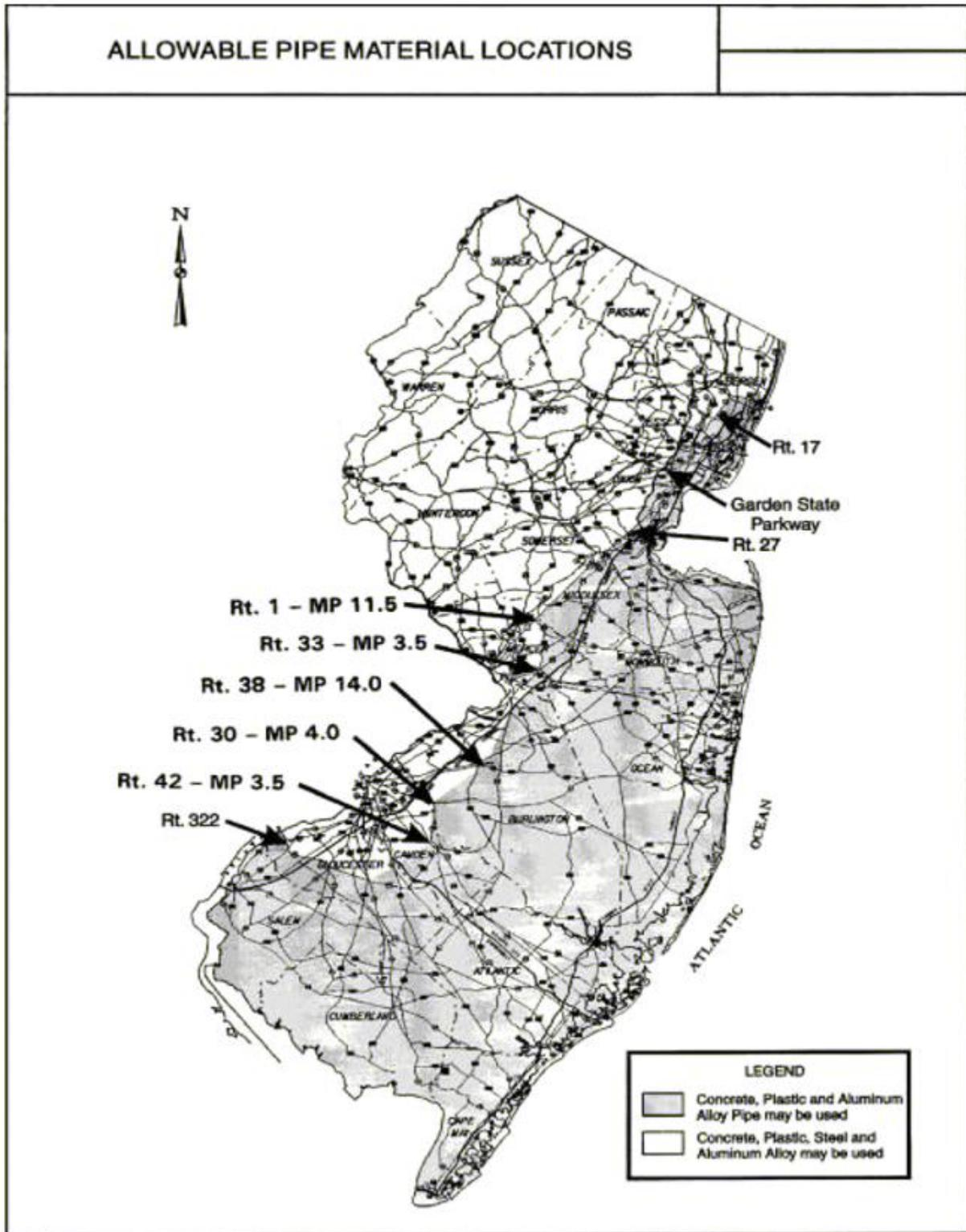
When alternate bid pipe materials are required, separate hydraulic calculations must be developed and submitted for each material considered (concrete, corrugated metal/aluminum alloy) using the respective roughness coefficients. The reason for exclusive use of a pipe material must be explained in the Drainage Report.
