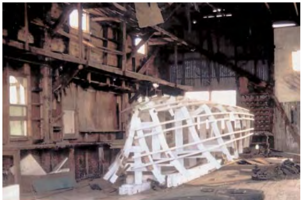
Atlantic City skiffs were built upside down over sturdy re-usable wooden forms. Carl Adams left this one in the Modern Boat Works shop when he retired in 1964. Besides the skiff form, several of his tools can be seen in the background [Source: New Jersey Department of Transportation].
