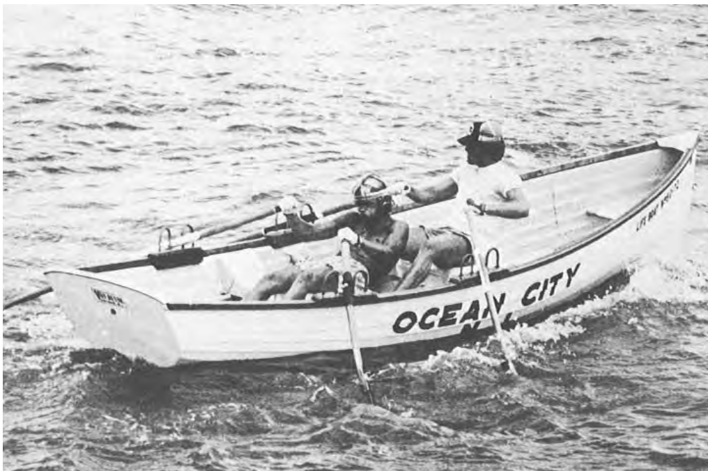
The usefulness of the skiff design for beach use is still evident. Here two Ocean City lifeguards are pulling in a modern fiberglass version of the traditional Atlantic City skiff, built in nearby Linwood [Source: The Sea Bright Skiff].
