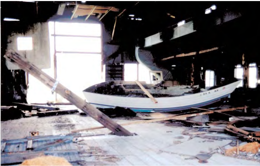
When Carl Adams closed his shop for the last time, he left behind not only his tools and raw materials but some unfinished work. Here a typical Jersey skiff sits on the shop floor, awaiting repair; the typical lapstrake planking is evident [Source: New Jersey Department of Transportation].
