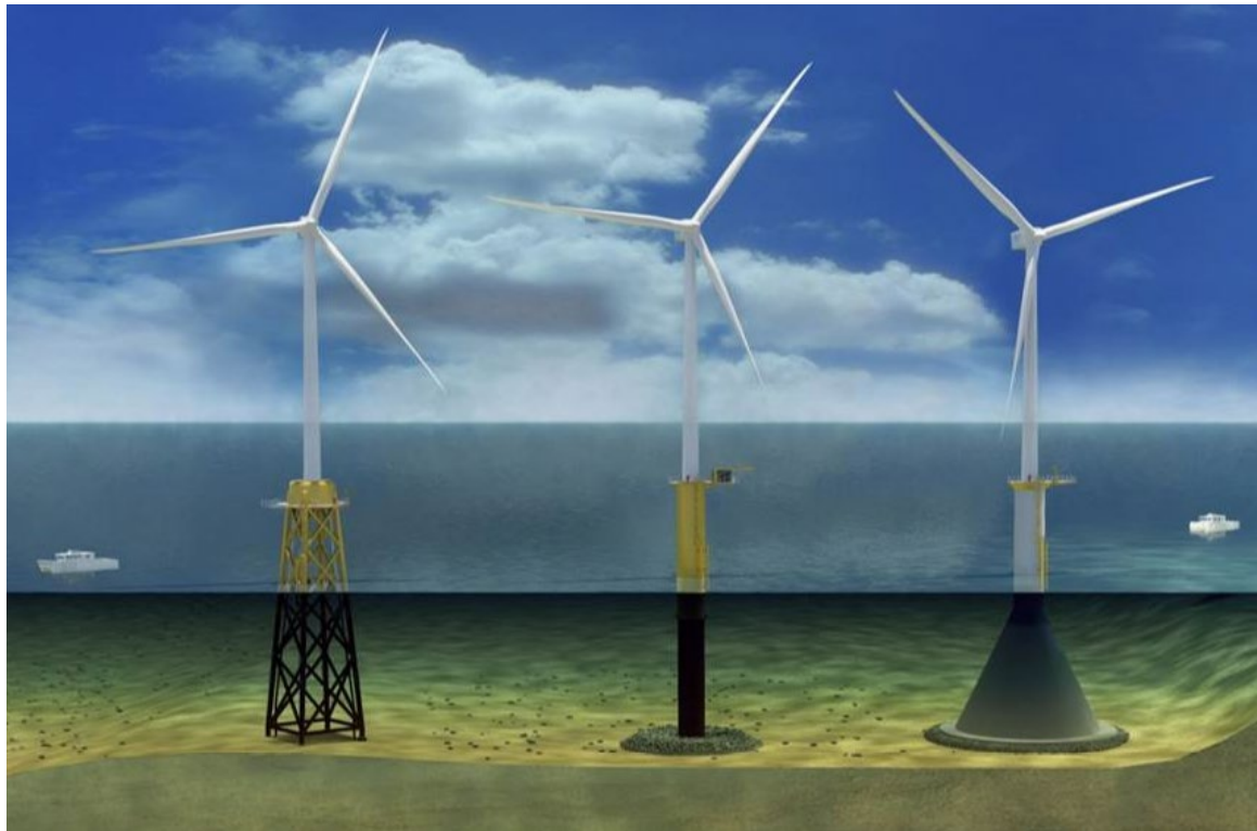
Figure 1: Foundation Concepts Including Jacket, Monopiles, and Gravity-based
