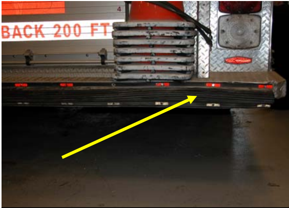
PHOTO 1: Shows rubber bladder component of the "BACKSTOP" system, and pre-existing impact damage near right corner area of rear step bumper of E-2. This is also believed to be the area where FF Stephens was struck.
