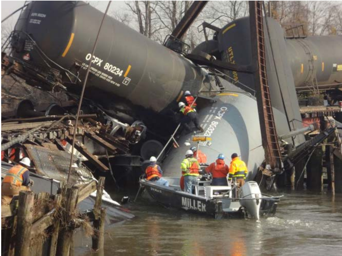
Figure 12. Personnel inspecting the breached tank car containing vinyl chloride liquid and vapor.
