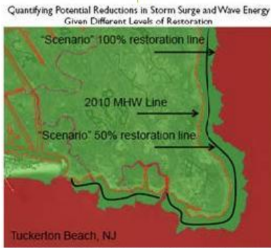
Figure 3-7: Wetlands Restoration, Tuckerton Beach, NJ. The efficacy and cost-effectiveness of nature-based risk reduction measures are being considered as potential solutions to reduce surge and flood risk. For example, by identifying potential wetland restoration scenarios, combined with dynamic modeling of the potential impact on wave energy and storm surge, the State can perform quantitative and qualitative analyses of the risk reduction provided by wetland restoration. This effort, undertaken by New Jersey in partnership with the Richard Stockton College of New Jersey, also allows for dynamic benefit-cost calculations. Source: State of New Jersey/The Richard Stockton College of New Jersey Partnership
