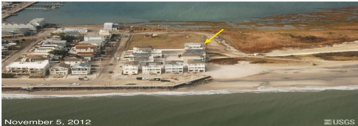
**Figure 28 - Storm waves and surge eroded the beach and exposed the seawall during Superstorm Sandy. Overwash of the seawall is indicated by sand deposited on the street. Low dunes on the eastern flank of the seawall were eroded. The yellow arrow in each image points to the same feature.**
