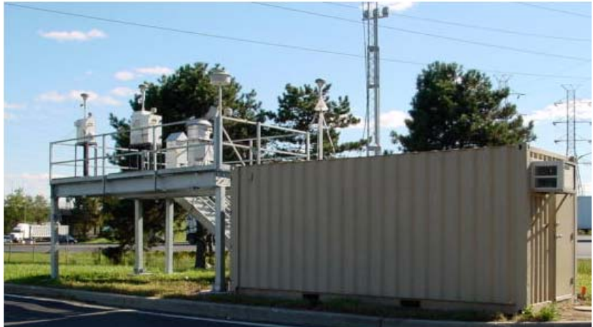
Figure 1: Ambient air monitoring trailer located at the Elizabeth Lab site
