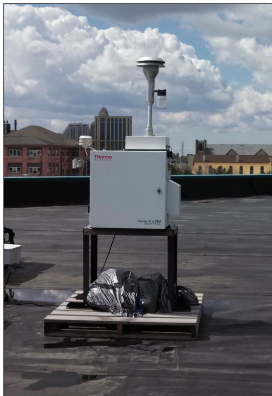
USEPA-approved manual PM 2.5 sampler on the roof of the Atlantic Cape Community College building in Atlantic City
