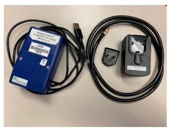
The aethalometer used in this project is a self-contained, pocket-sized instrument with flow control, data storage and battery. Aethalometers similar to this are used by air quality monitoring programs, public health protection agencies, research laboratories and community groups.
