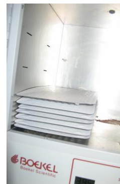
Figure 6-8. On the far left we have an example of the Petri dishes in the incubator. The center picture is of the two incubators and the IDEXX sealer. On the right there is a stack of IDEXX trays being incubated.
