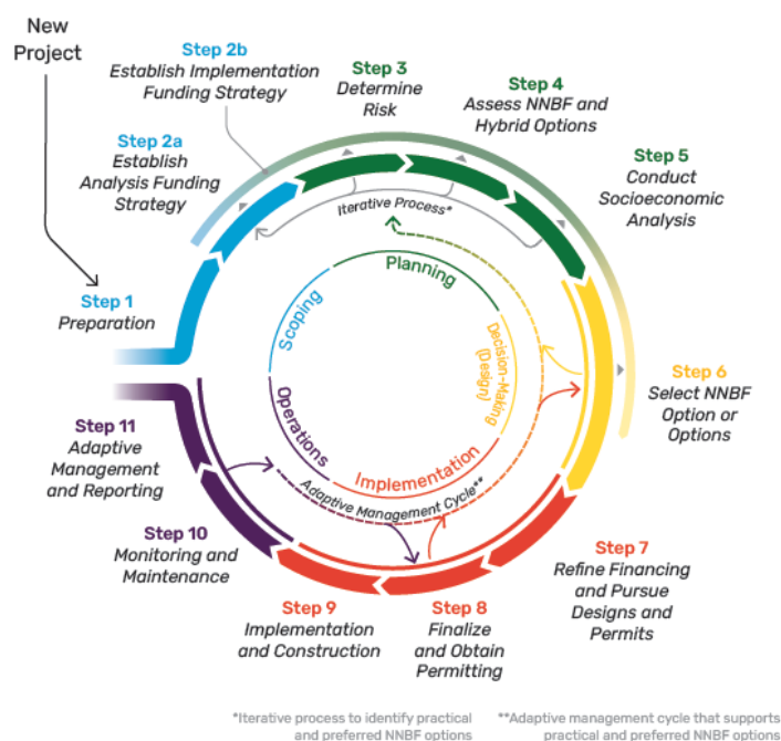
Figure 4: IGNNBF process for identifying and implementing the preferred NNBF alternative
