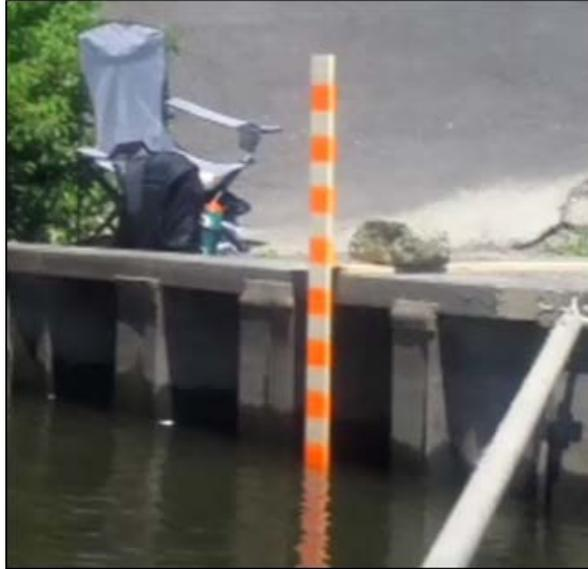
Figure 4: Visual Wake Measurement near a Bulkhead
