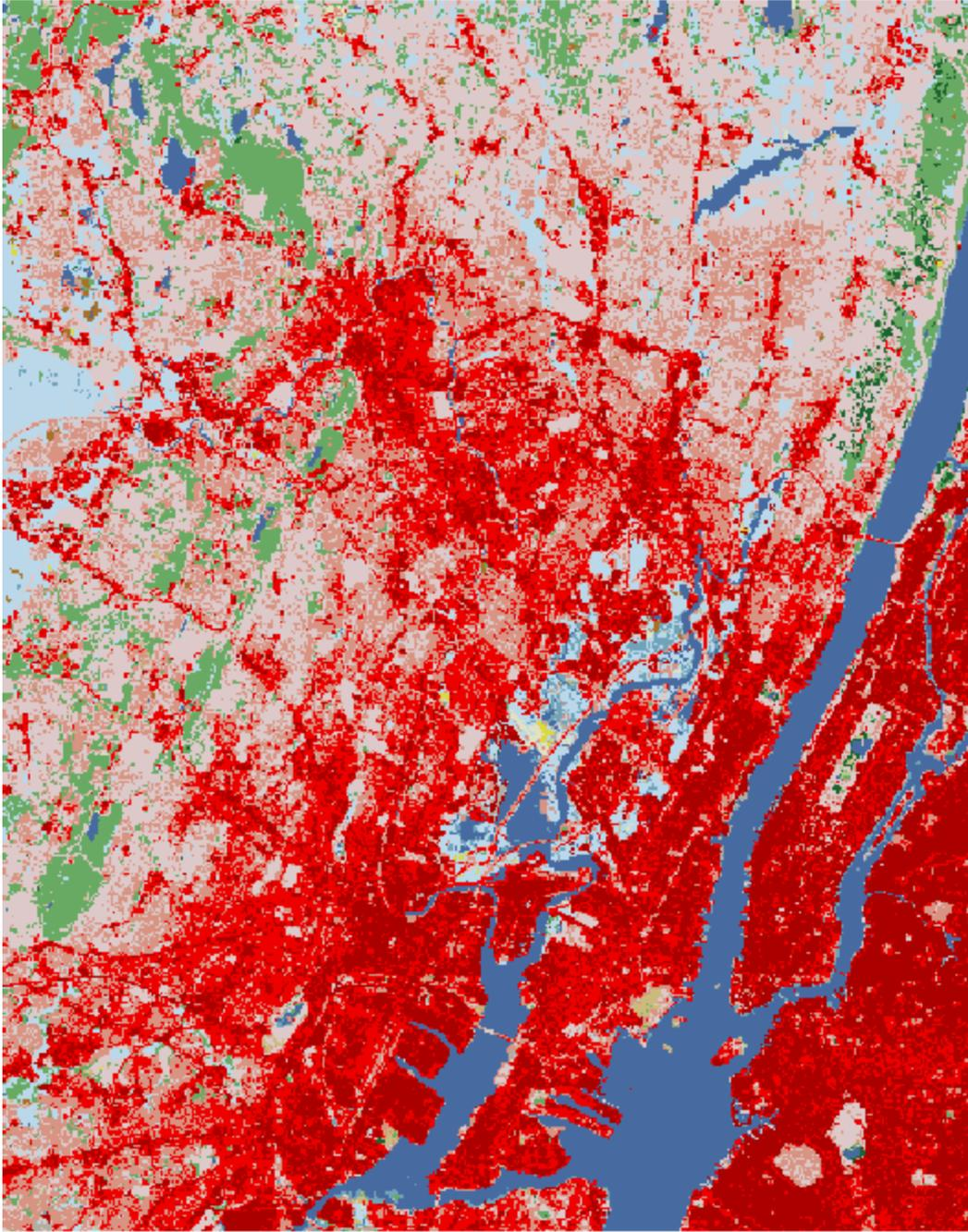
Figure 6 Land use classes in the computational domain (see Table 1 for the color code, description for each land use class and the corresponding Manning's  $n$  values).
