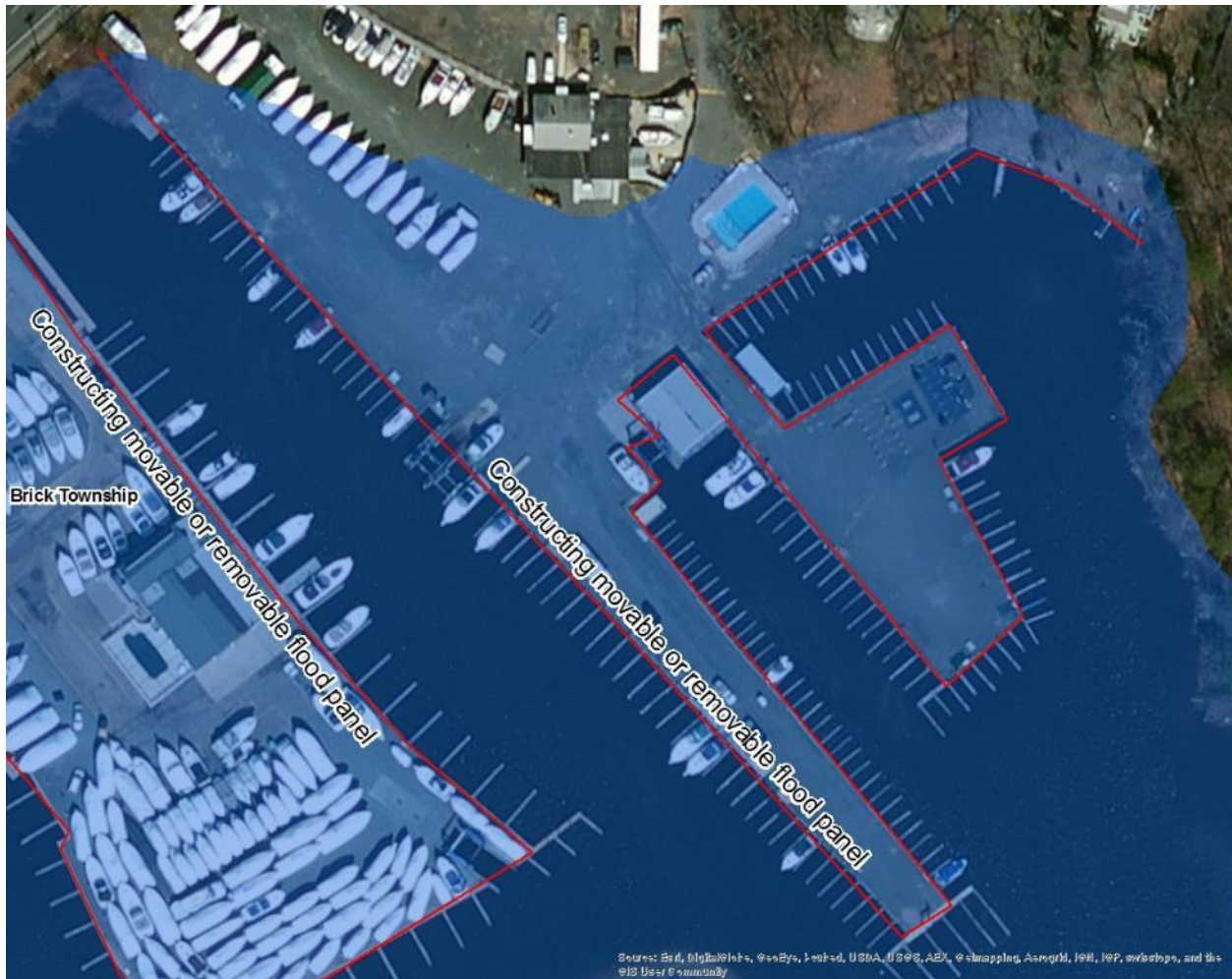
Fig. 4.6.2 Constructing Movable or Removable Flood Panels to Protect Marina Area
