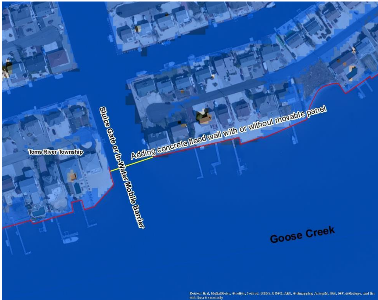
Fig. 4.10.1 Constructing Sluice Gate or In-water Barrier at Lagoon Ends: (1) Yellow line represents Sluice Gate or In-water Barrier, (2) Red line represents bulkhead with or without movable flood panels.
