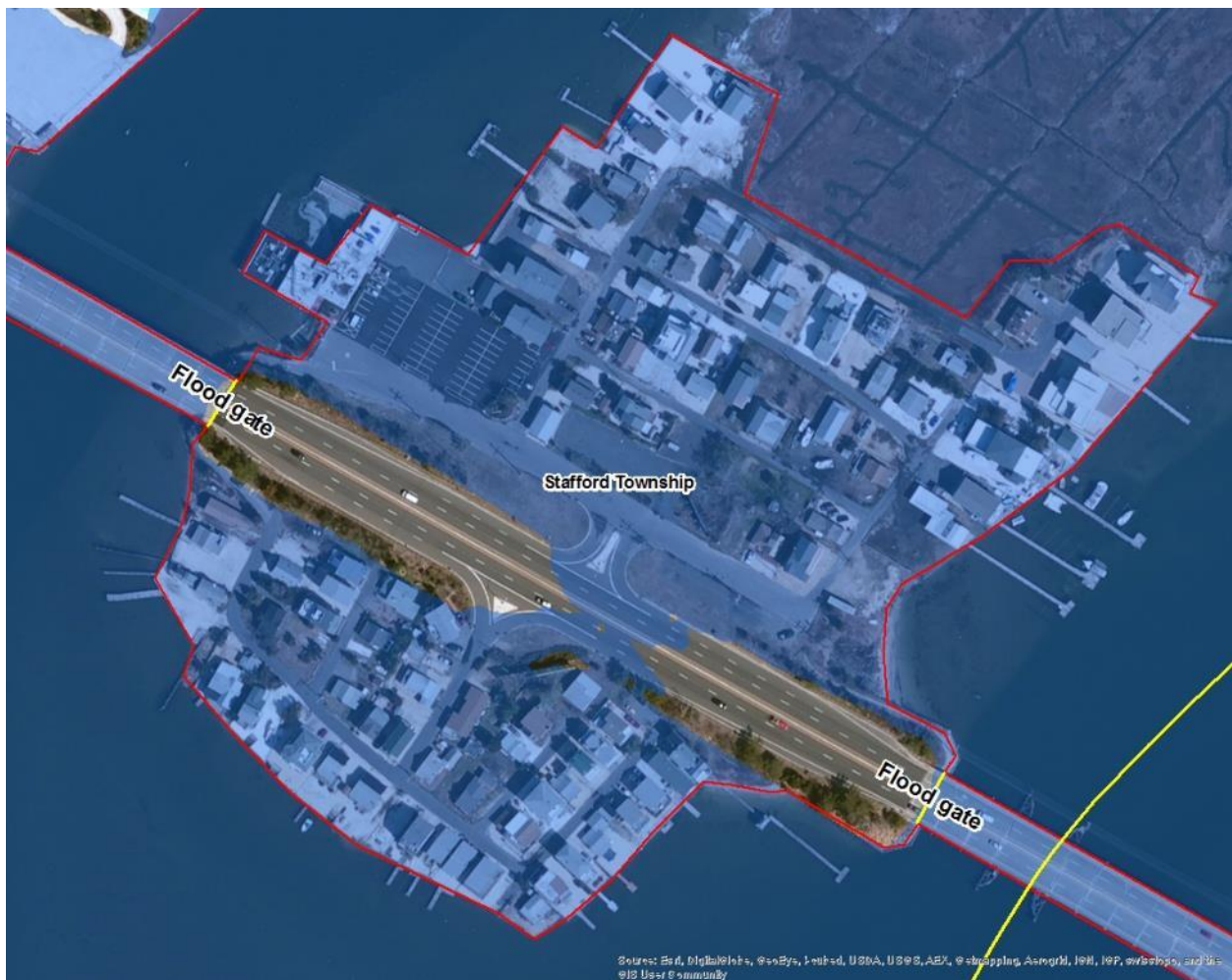
Fig. 4.11.1 Constructing a Flood Gate to Protect the Closed Area: (1) Yellow line represents flood gate, (2) Red line represents bulkhead or levee.
