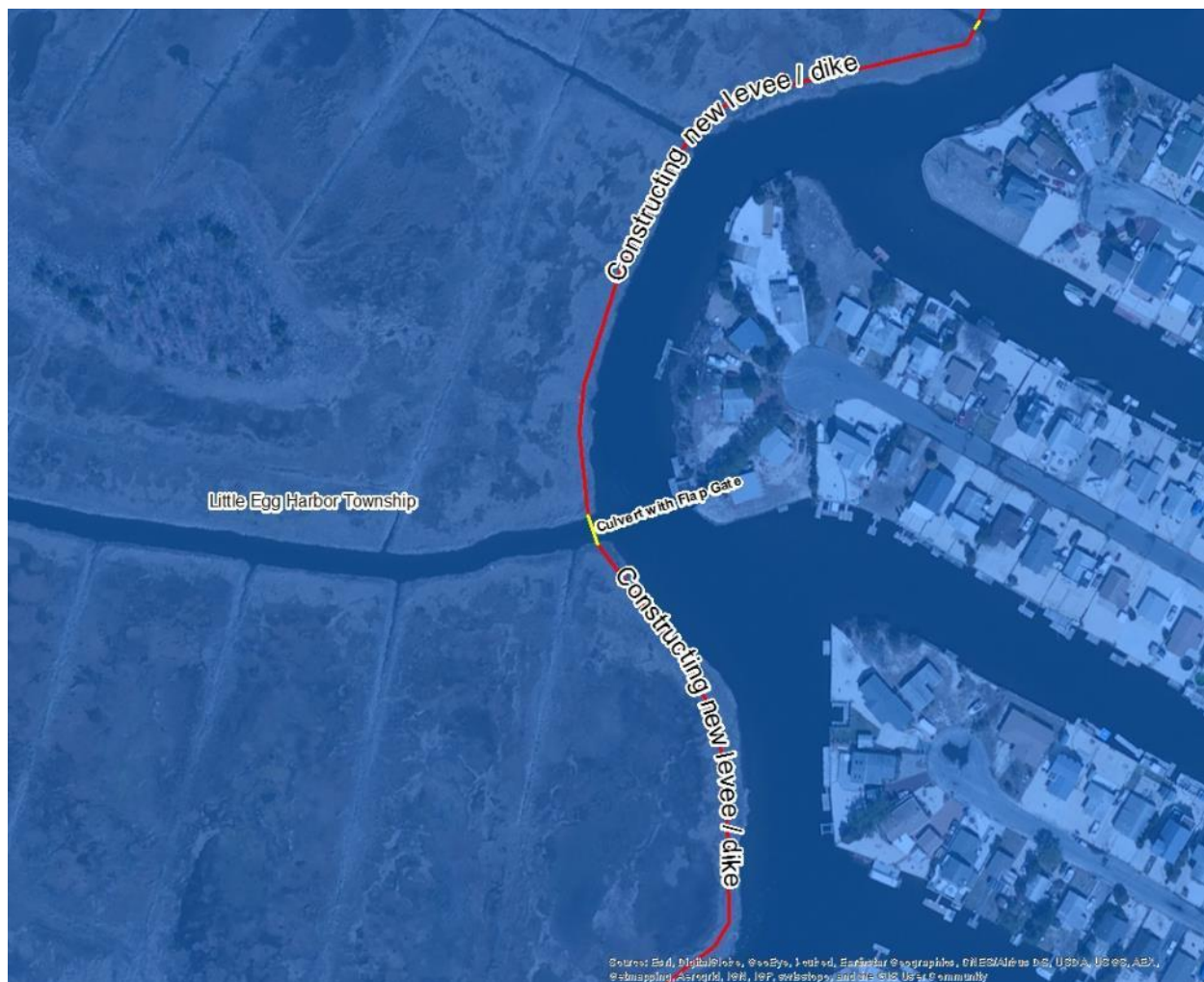
Fig.4.7.2 Constructing a New Levee and Culvert with Flap Gate
