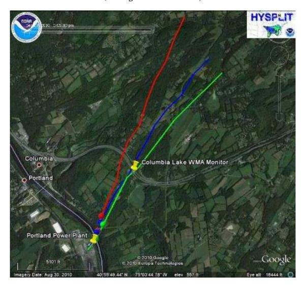
Red Line = 10 meter above ground trajectory (approximate monitor height)
