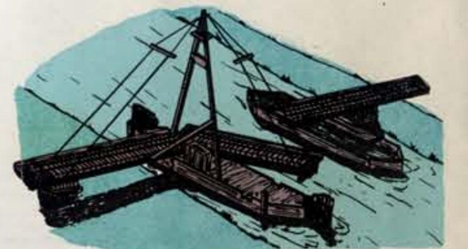
A "sheer leg" bridge. The canal was crossed by over 60 bridges. A few were lift bridges, many were off center swing bridges, and a number were the unusual "A frame" or "sheer leg" bridges.
