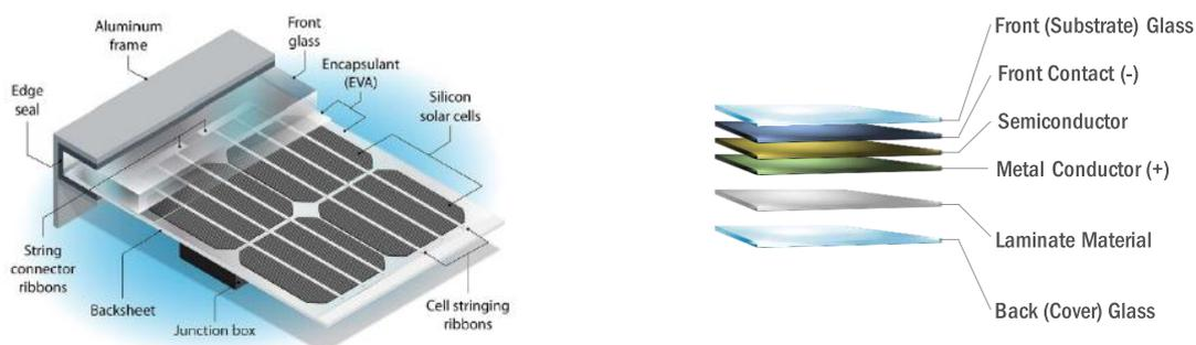
Figure 1: c-Si (left) [1] and thin film (right) [13] PV module components
