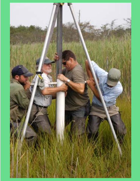
Figure 2. Tripod and pulley system used to retrieve push-piston cores from marshes in Barnegat Bay.
